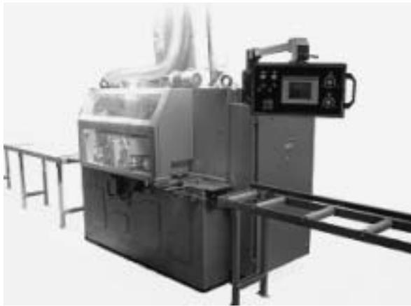
**Figure 1** A testing stand for high-speed milling
