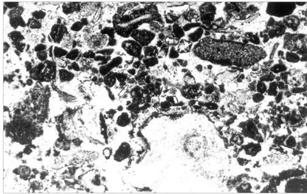
Fig. 14 A photomicrograph of bioclastic–intraclastic–peloidal grainstone with coarse bioclasts; lithofacies C, Breze column, 13x.
