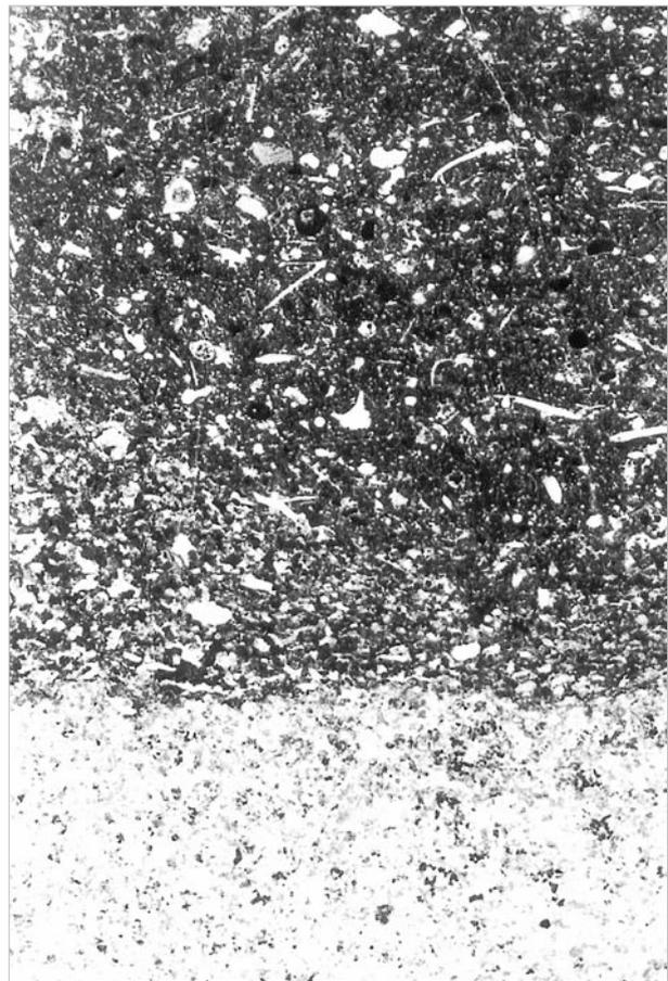
Fig. 8 A photomicrograph of the irregular contact of a diagenetic chert nodule (light grey) and peloidal-bioclastic wackestone/packstone; lithofacies B<sub>1</sub>, Mala Javornica column, 6.5x.
