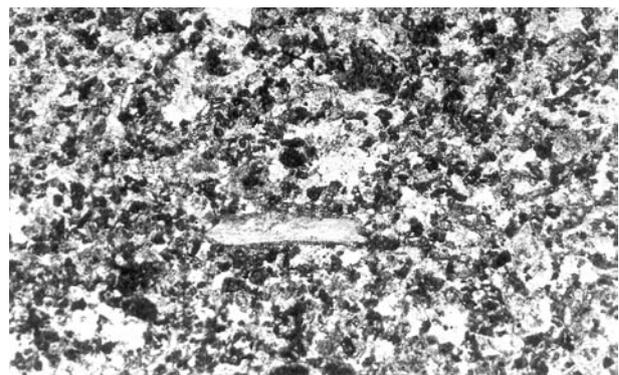
Fig. 12 A photomicrograph of fine-grained, relatively well-sorted bioclastic-intraclastic-peloidal packstone/grainstone; lithofacies B<sub>2</sub>, Breze column, 10.5x.
