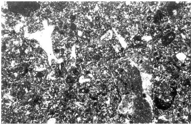
Fig. 13 A photomicrograph of bioclastic–intraclastic–peloidal packstone with coarse bioclasts of molluscs and pelagic forms including *Saccocoma* sp.; lithofacies B<sub>2</sub>, Tuk column, 8.5x.
