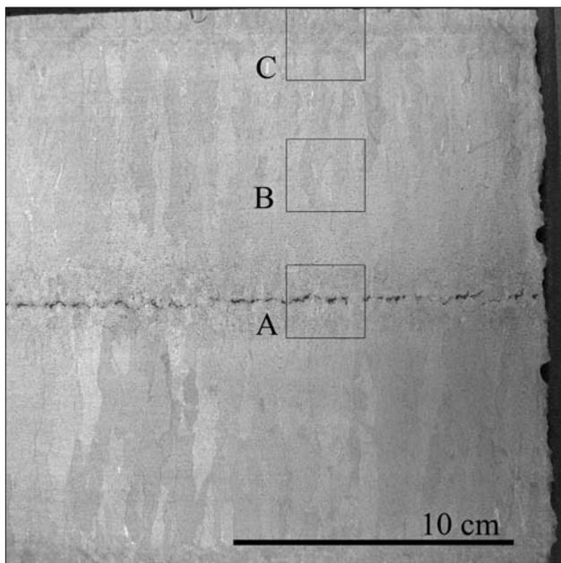
Figure 2. As-cast sample taken from slab perpendicular to casting direction.
