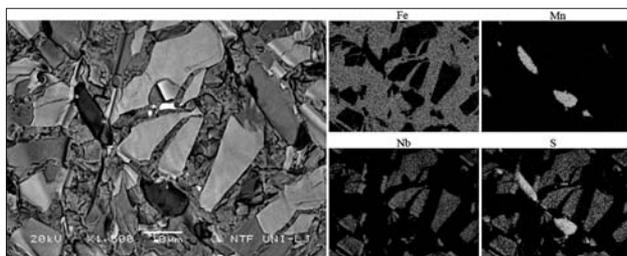
Figure 4. EPMA mapping of Nb(C, N) and MnS particles.
