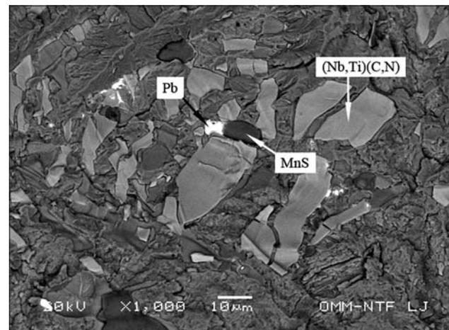
Figure 3. SEM fractograph of the reduction of area specimen. Analysed particles are marked with arrows, EDXS analyses are presented in Table 2.
