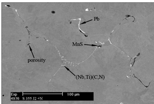
Figure 5. SEM picture of degenerated eutectic in form of "Chinese script" from the sample A of the as cast slab.
