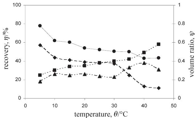
Fig. 3 – Partition result for plasmid DNA in 15:22 ATPS ( $w = 15$  % PEG-300,  $w = 22$  % phosphate and  $w = 40$  % lysate) with respect to system temperature: (◆) top phase, (■) bottom phase, (▲) interface, (●) volume ratio
