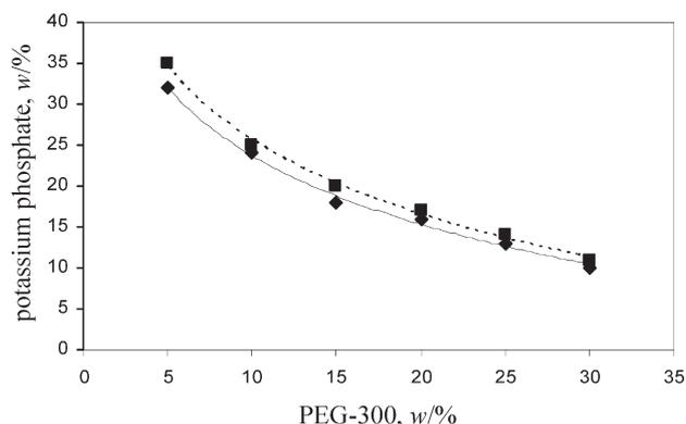
Fig. 1 – Phase diagram for PEG-300/ $\text{K}_2\text{HPO}_4$ : (◆) crude binodial with  $w = 40$  % lysate and (■) clean ATPS. Biphasic regions are to the right of the binodial curve.
