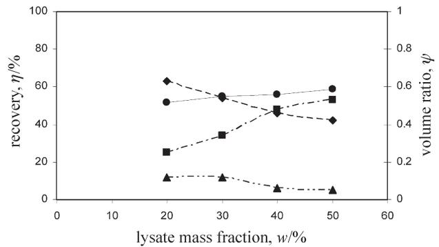
Fig. 4 – Partition result for plasmid DNA in 15:22 ATPS ( $w = 15$  % PEG-300,  $w = 22$  % phosphate and  $w = 40$  % lysate) with respect to lysate fraction at  $20$  °C: (◆) top phase, (■) bottom phase, (▲) interface, (●) volume ratio
