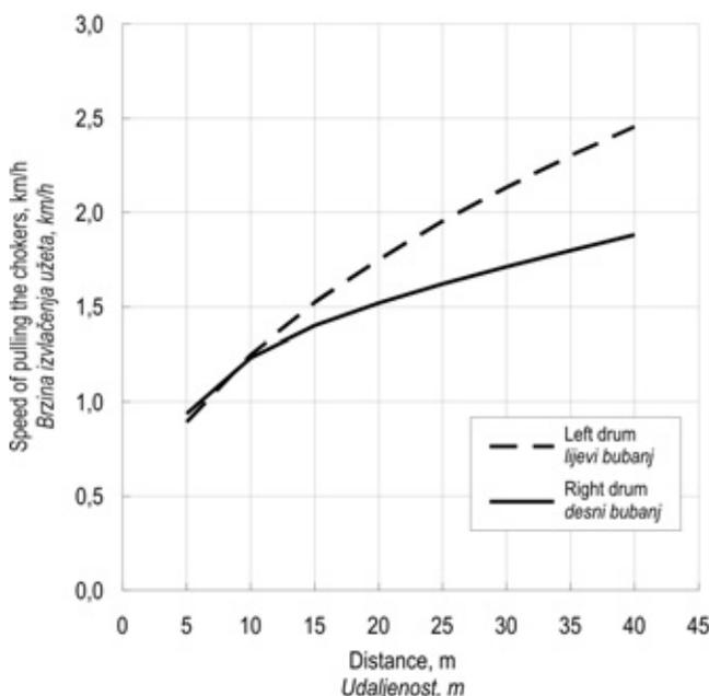
**Figure 6** Speeds of pulling the choker of the left and right drum**Slika 6.** Brzine izvlačenja užeta lijevoga i desnoga bubnja
