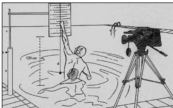
Figure 1. In-water vertical jump. Vertical pole consists of two parts (a and c). Part (c) could be extended upwards by adjusting the total height of the pole. a. Lower part of vertical pole. b. Vertical pin sliding into holes made on the upper pole. c. Upper part of vertical pole. d. A piece of string with a small weight attached to its end (plumb line).
