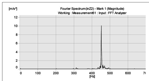
Figure 10. Accelerations dependent on frequencies bearing L4, 1100 rpm
