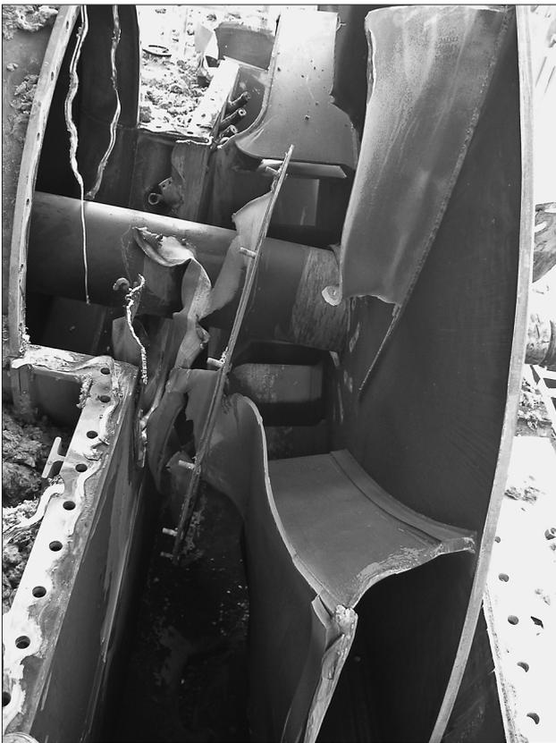
Figure 7. Damaged rotating wheel and covering steel sheet
