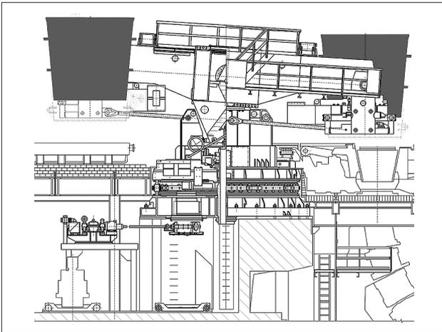
Figure 1. Casting pedestal with pans
