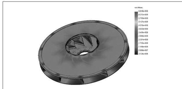
Figure 8. Strains and equivalent stresses in rotating wheel
