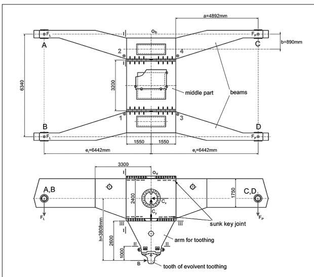
Figure 2. Traverse of casting pedestal
