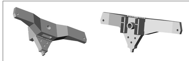
Figure 3. Computational model of casting pedestal traverse
