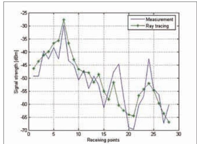
Figure 12. Comparison of the results between the measurement and raytracing model for AP2
