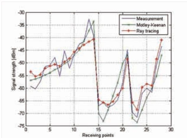
Figure 16. Comparison between signal strength prediction using measurement, ray tracing and Motley-Keenan model for AP3
