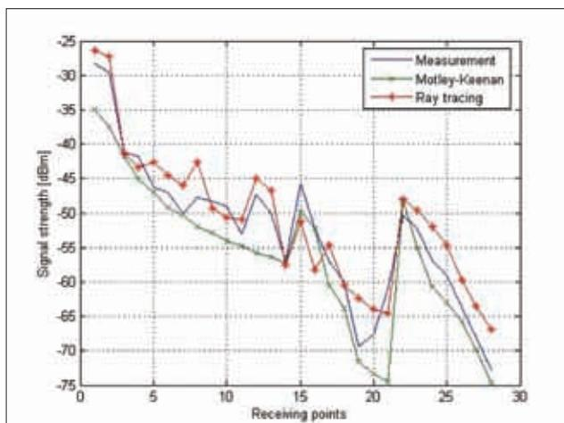
Figure 14. Comparison between signal strength prediction using measurement, ray tracing and Motley-Keenan model for AP1
