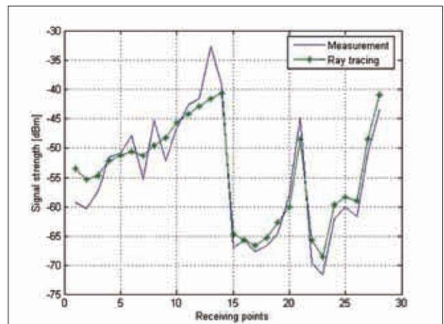
Figure 13. Comparison of the results between the measurement and raytracing model for AP3
