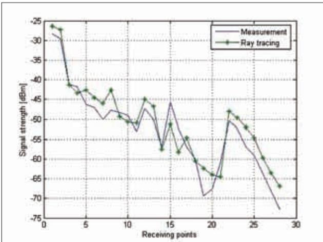
Figure 11. Comparison of the results between the measurement and raytracing model for AP1
