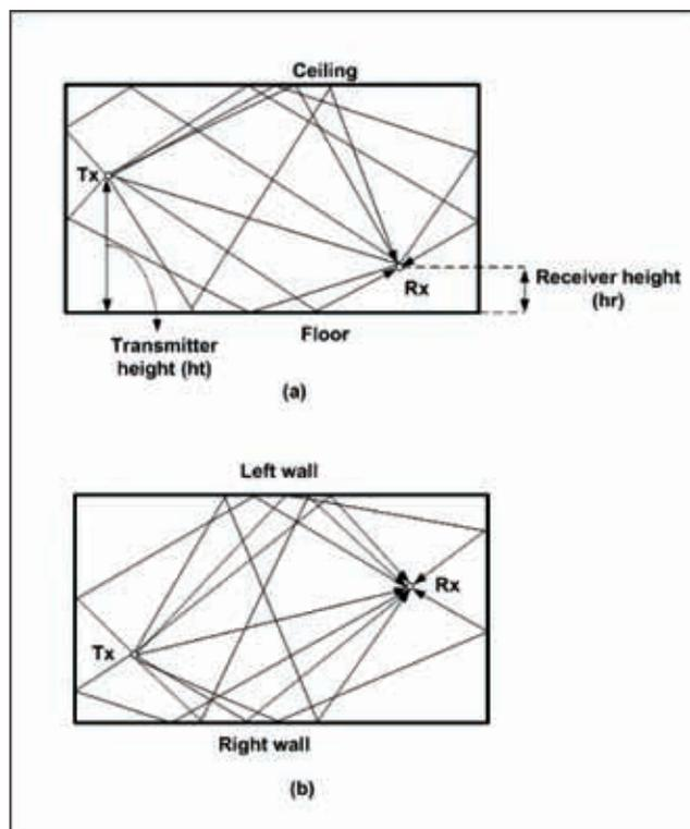
Figure 10. Propagation geometry, paths of the chosen rays: a) vertical plane, b) horizontal plane
