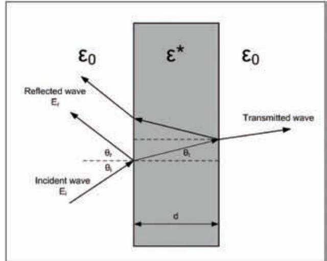
Figure 2. Reflection and transmission mechanism in slab
