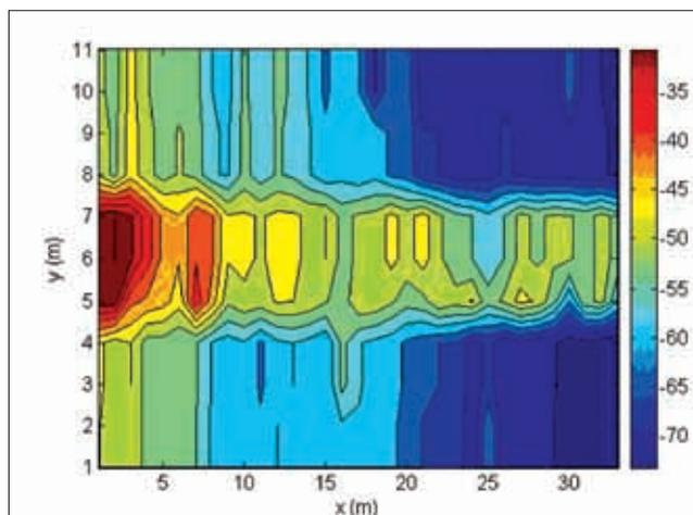
Figure 9. Contour map of the measured receiver power strength for access point AP1
