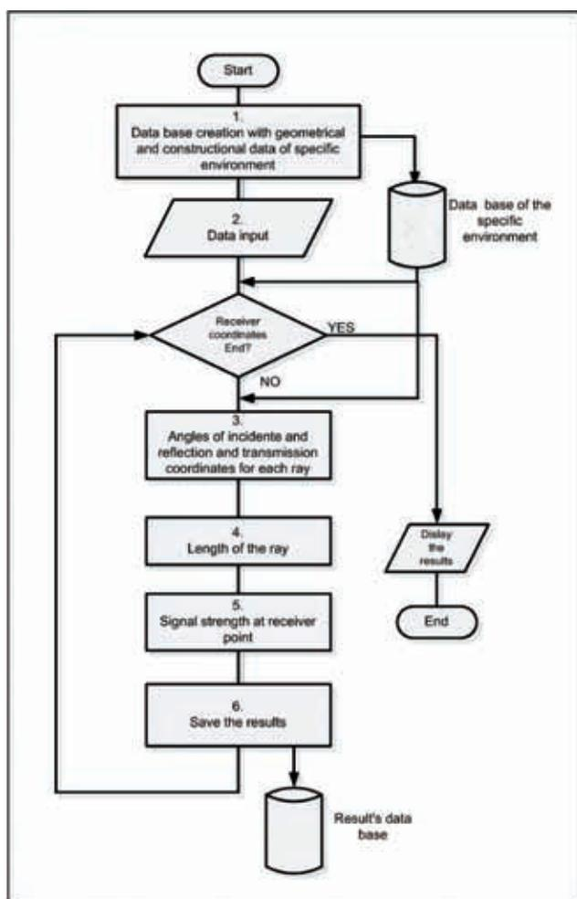
Figure 3. Algorithm for ray tracing model
