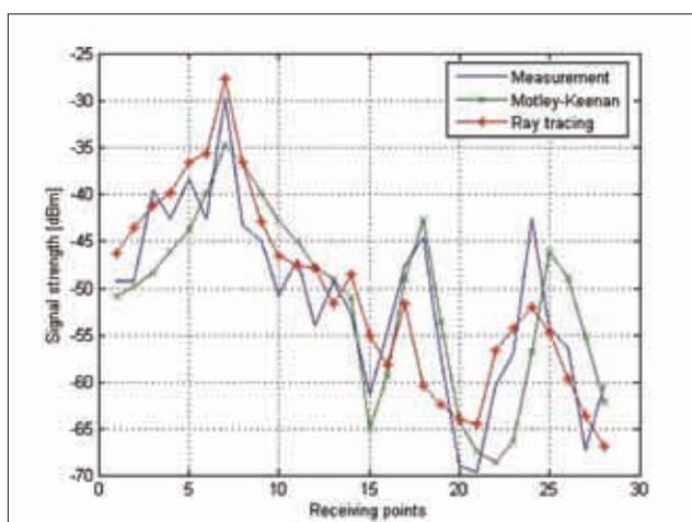
Figure 15. Comparison between signal strength prediction using measurement, ray tracing and Motley-Keenan model for AP2
