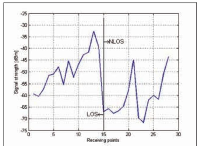
Figure 8. Signal propagation for the access point AP3
