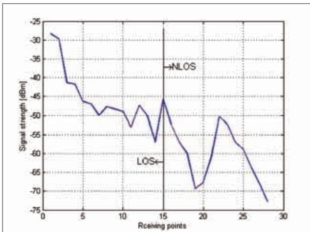
Figure 6. Signal propagation for the access point AP1
