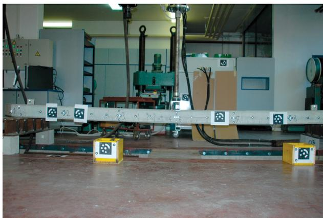
Fig. 1. *Prefabricated prestressed concrete plate with measured marks.*
