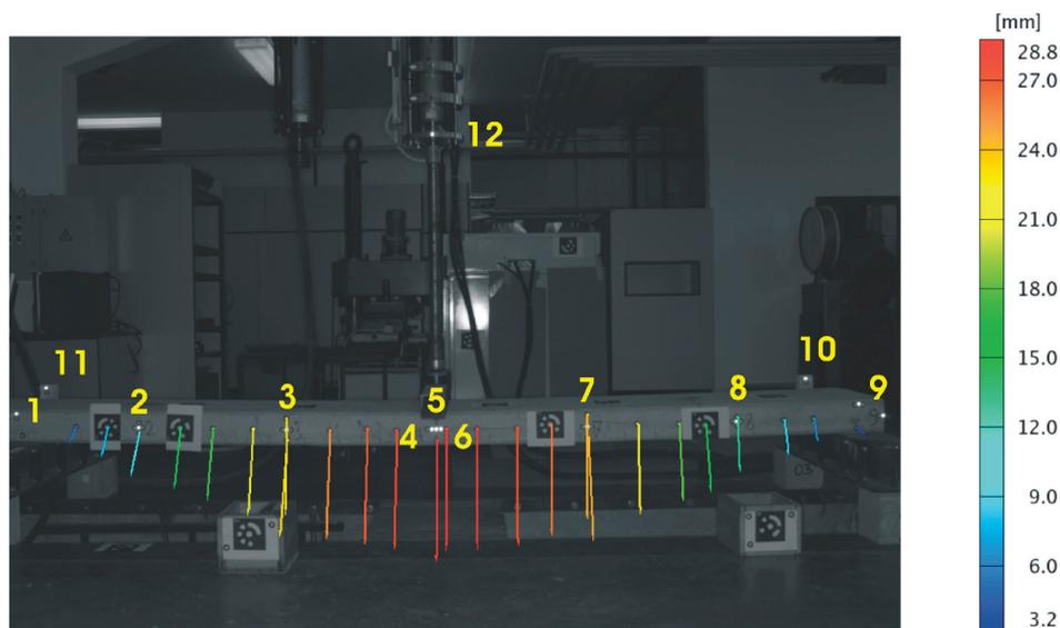
Fig. 5. Reference points, coded marks, scale bars and displacement vectors of a concrete plate.
