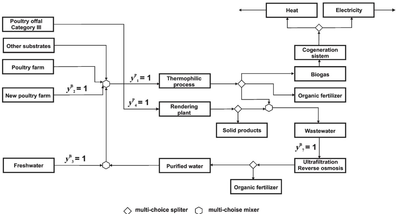
Fig. 4 – Optimal solution for the industrial case study of biogas production in a combined thermophilic process, and a rendering plant
