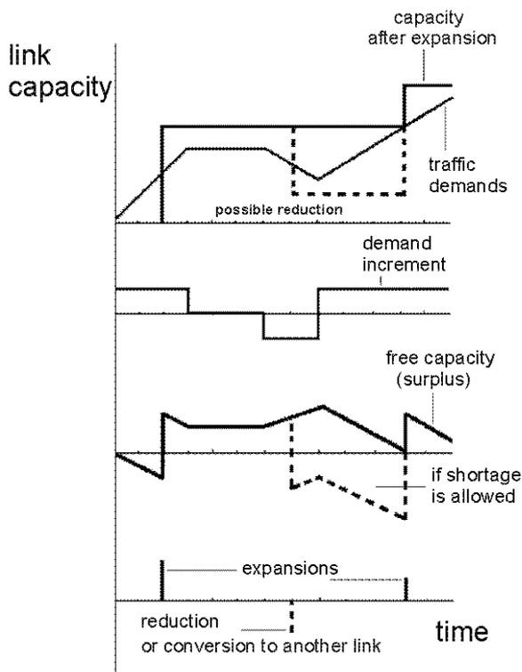
Figure 1 Capacity planning for only one capacity type over the finite time period
