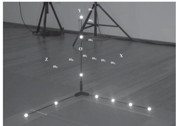
Figure 1. Wand calibration. First calibration step – an initialization of the camera parameters. Marker distances [mm] with respect to the triad origin O: X-axis  $m_1=150$ ,  $m_2=300$ ,  $m_3=450$ ,  $m_4=600$ ; Y-axis  $m_5=150$ ,  $m_6=450$ ,  $m_7=600$ ; Z-axis  $m_8=300$ ,  $m_9=600$ .
