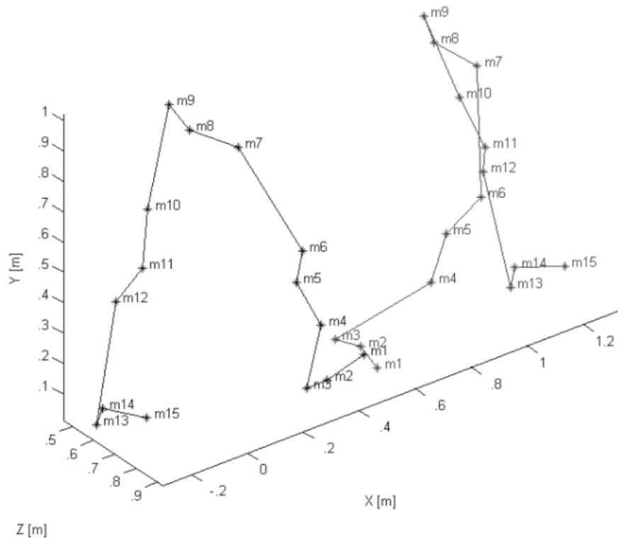
Figure 4. 3D reconstruction of markers at the beginning of the stance phase (left) and at the end of the stance phase (right). Markers m1 to m15 were set for gait analyses according to the Helen Hayes protocol as described by Vaughan, Davis and O'Connor (1999).
