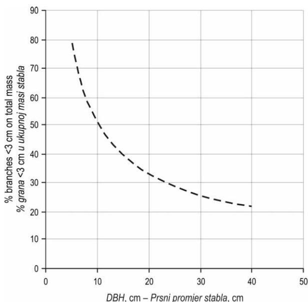
**Fig. 1** Incidence of the branch portion (diameter <3 cm) on the total tree mass, weighted with portable scales
