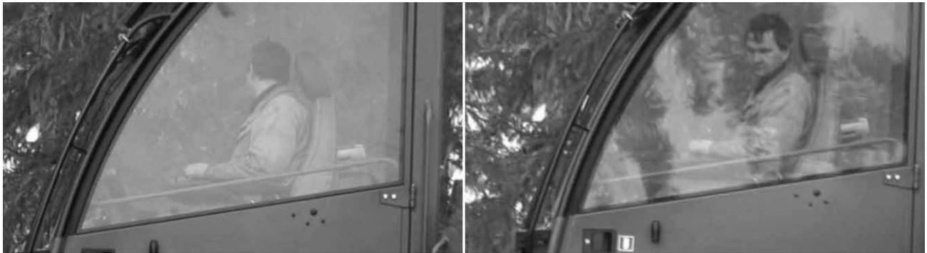
**Fig. 2** Uncomfortable work postures when operating a harvester without a rotating cab
