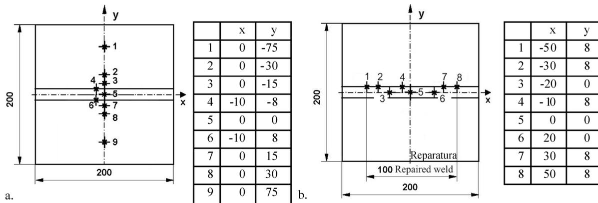
**Figure 1.** Location of the residual stresses measurements on the welded plates, (a) for three different welding conditions and (b) for repair welding
