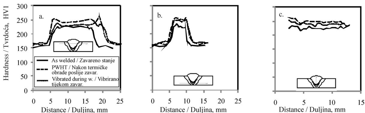
**Figure 3.** Comparison of Vicker's hardness profile on the T.I.M.E. welded joints in three different conditions (as welded, PWHT and vibrated during welding) (a) weld cap, (b) root, (c) WM
