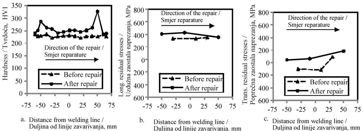
Figure 8. Results of hardness and residual stress measurement (a) Hardness, (b) Longitudinal residual stresses (c) Transverse residual stresses
