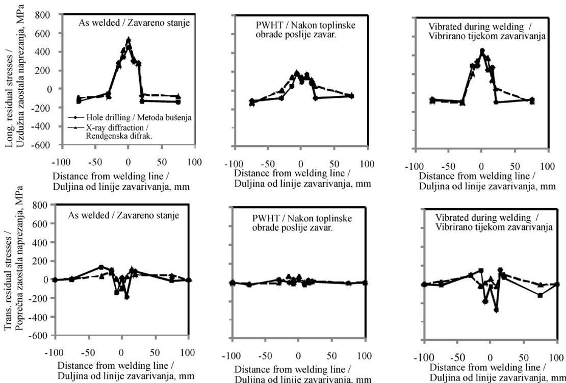
Figure 4. Comparison of the hole drilling and X-ray diffraction method using longitudinal and transverse residual stresses on the SAW welded joints in three different conditions
