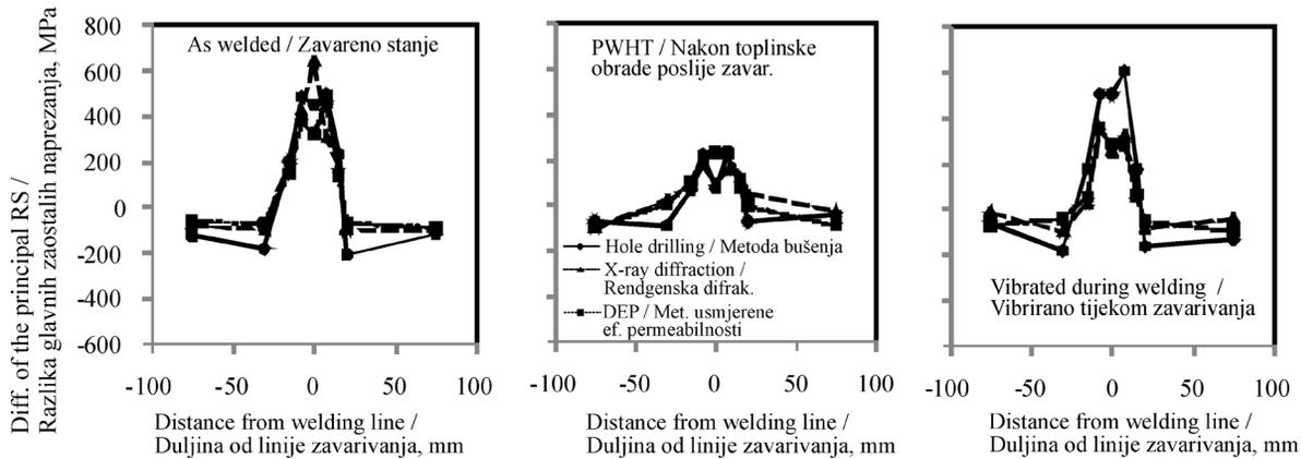
Figure 6. Comparison of the hole drilling, X-ray diffraction and DEP method using differences of the principal residual stresses on the SAW weld joints in three different conditions
