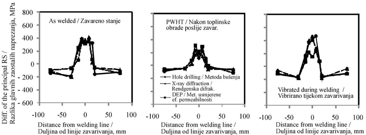
Figure 7. Comparison of the hole drilling, X-ray diffraction and DEP method using differences of the principal residual stresses on the T.I.M.E. weld joints in three different conditions
