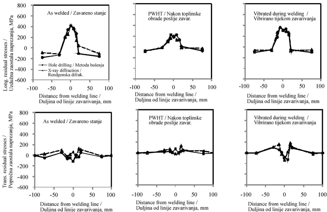
Figure 5. Comparison of the hole drilling and X-ray diffraction method using longitudinal and transverse residual stresses on the T.I.M.E. welded joints in three different conditions
