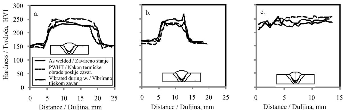
**Figure 2.** Comparison of Vicker's hardness profile on the SAW welded joints in three different conditions (as welded, PWHT and vibrated during welding) (a) weld cap, (b) root, (c) WM
