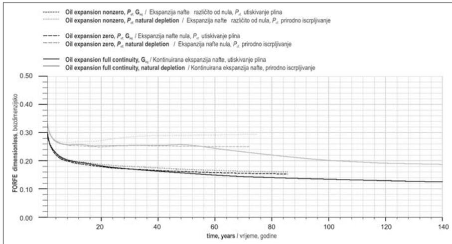
**Fig. 7. Impact of capillary continuity on oil expansion mechanism**
