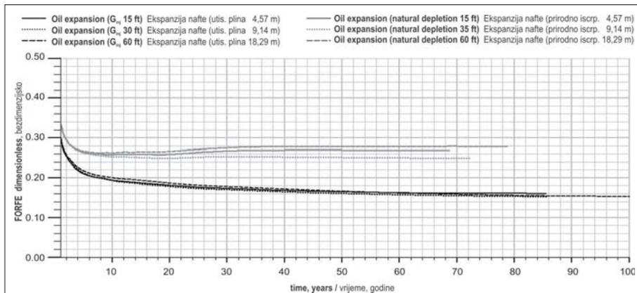
Fig. 3. Effect of matrix blocks height on oil expansion mechanism
