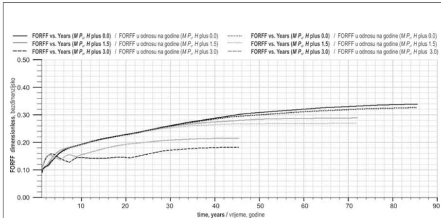
**Fig. 8. Impact of capillary continuity on gravity drainage mechanism of three different matrix capillary pressure cases**
