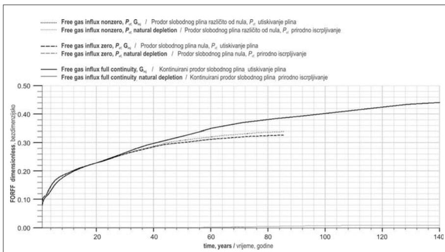
**Fig. 6. Impact of capillary continuity on gravity drainage mechanism**
