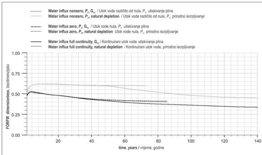
**Fig. 5. Impact of capillary continuity on water imbibition mechanism**
