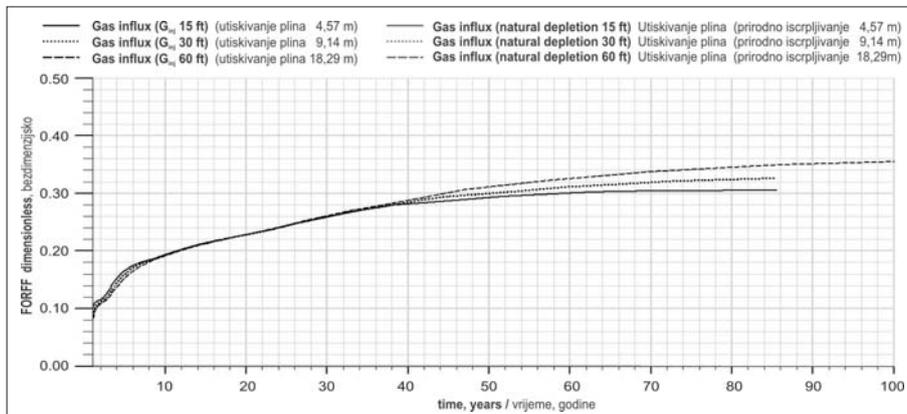
Fig. 4. Effect of matrix blocks height on gravity drainage mechanism
