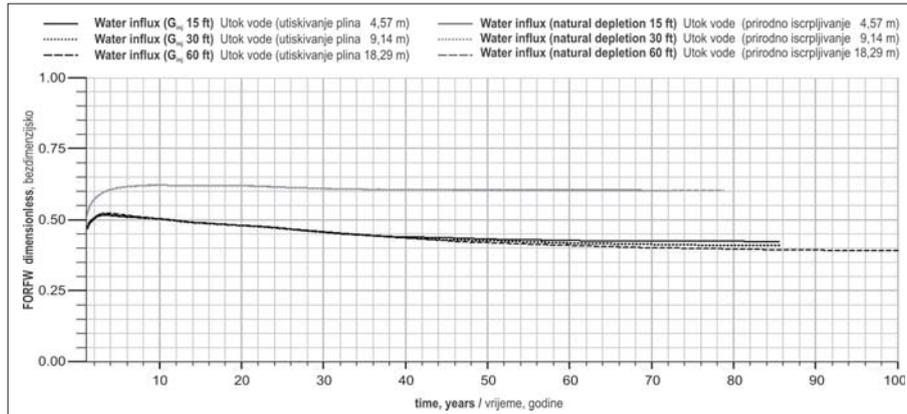
Fig. 2. Effect of matrix blocks height on water imbibition mechanism
