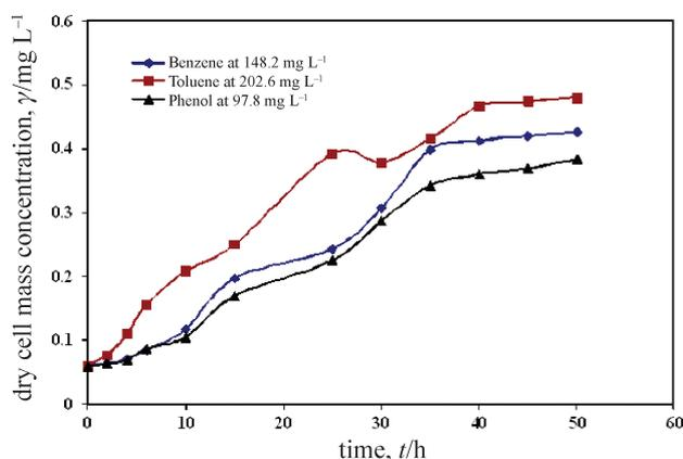
Fig. 3 – Biodegradation and cell growth at inhibition concentrations of benzene, toluene and phenol
