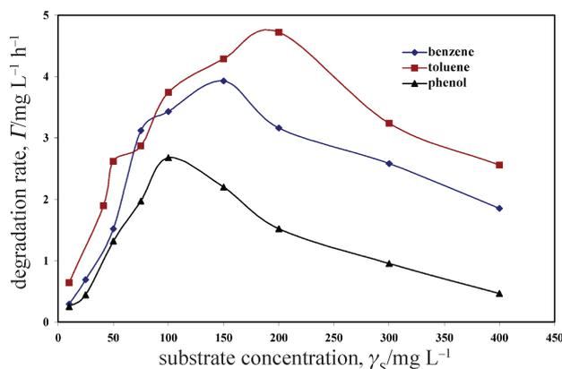
Fig. 2 – Effects of substrate concentration on degradation rate of benzene, toluene and phenol
