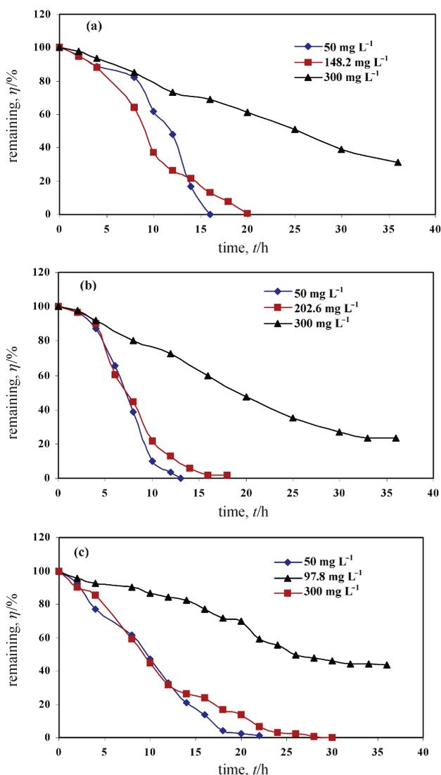
Fig. 4 – (a) Degradation rate profile of benzene in terms of percentage remaining with time (b) degradation rate profile of toluene in terms of percentage remaining with time (c) degradation rate profile of phenol in terms of percentage remaining with time
