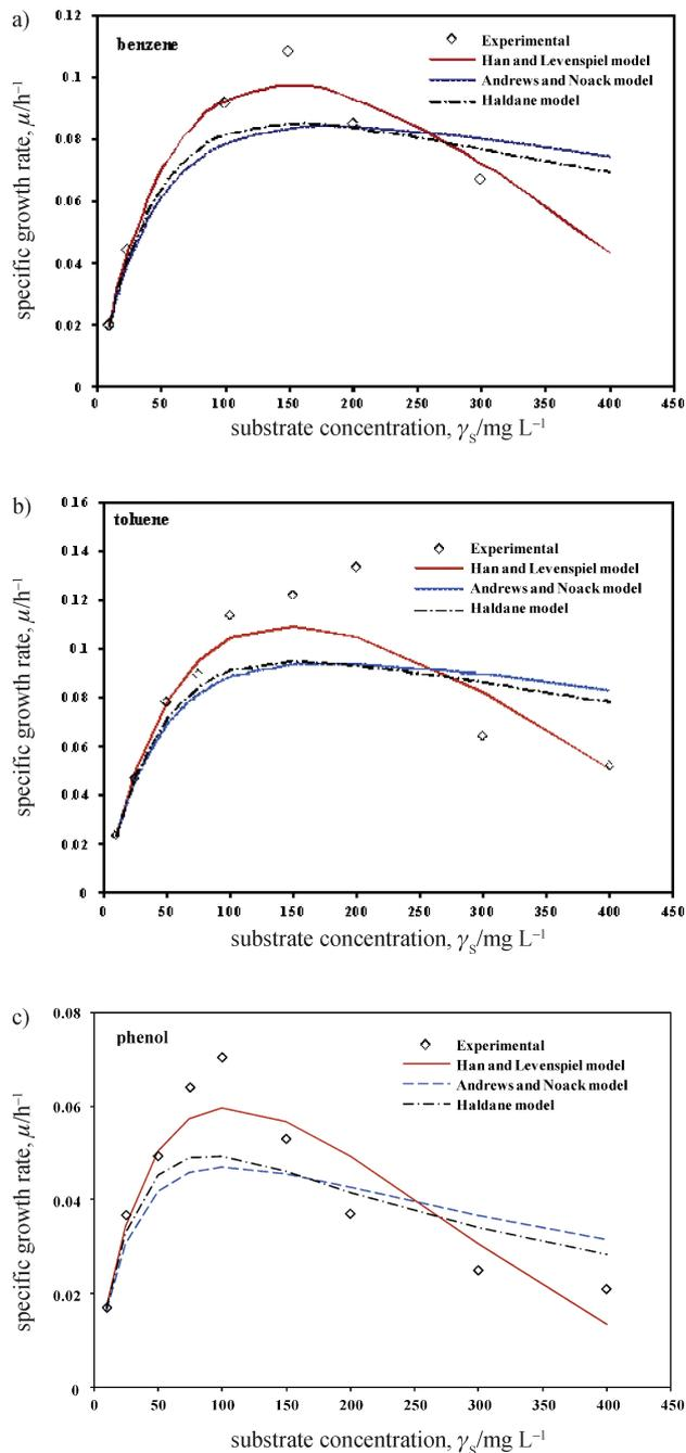
Fig. 6 – Experimental and model predicted profiles of specific growth rate for (a) benzene (b) toluene (c) phenol
