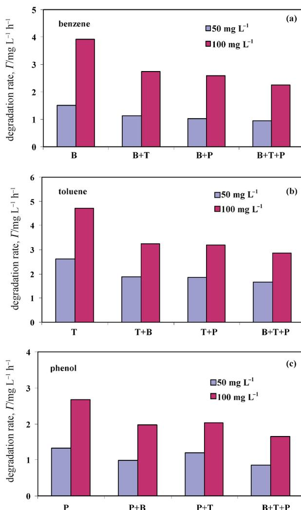
Fig. 5 – Substrate interaction in binary and three-component mixture (a) effects of single substrate and mixture of toluene and phenol on benzene biodegradation; (b) effects of single substrate and mixture of benzene and phenol on toluene biodegradation; (c) effects of single substrate and mixture of benzene and toluene on phenol biodegradation. Substrate interaction shows at  $50 \text{ mg L}^{-1}$  and  $100 \text{ mg L}^{-1}$  of each component.
