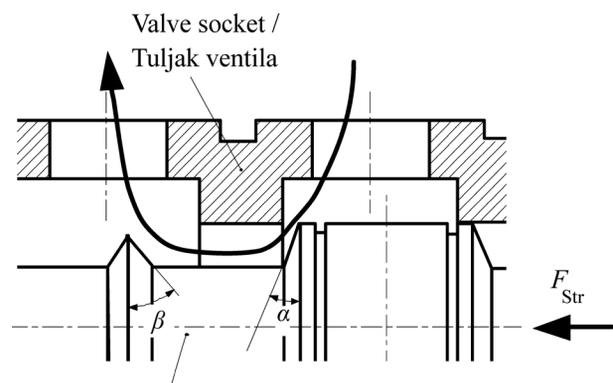
Figure 3. Spool geometry of the inlet edge
