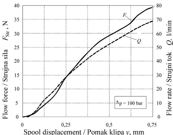
**Figure 8.** Flow force and the fluid flow, non-compensated spool,  $\Delta p = 100$  bar, the whole valve (P- > B- > A- > T)
