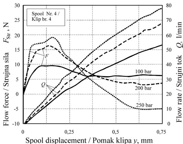
**Figure 12.** Flow-force measuring results, spool Nr. 4, the whole valve (P- > B- > A- > T)
