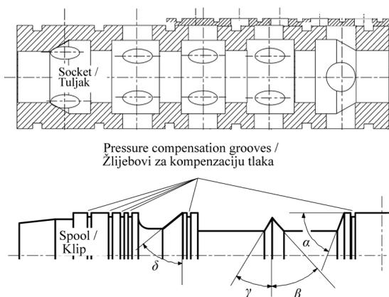
**Figure 5.** Valve socket and spool (flow force compensated)
