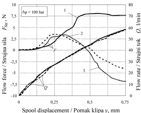
**Figure 9.** Flow force and the fluid flow, compensated spool (Nr. 1 – 3),  $\Delta p = 100$  bar, the whole valve (P- > B- > A- > T)
