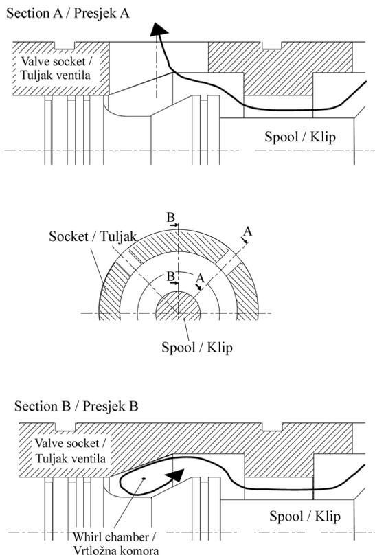
**Figure 4.** Spool and valve socket geometry of the outlet edge
