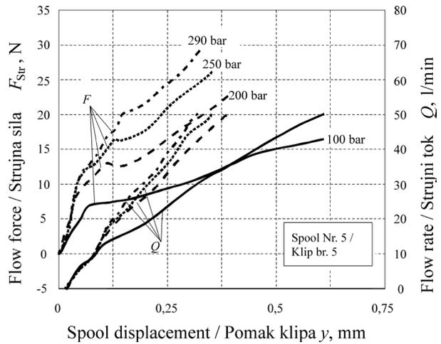
**Figure 16.** Force-force spool stroke and flow-rate spool stroke characteristics, spool Nr. 5, modified valve socket, the whole valve (P- > B- > A- > T)
