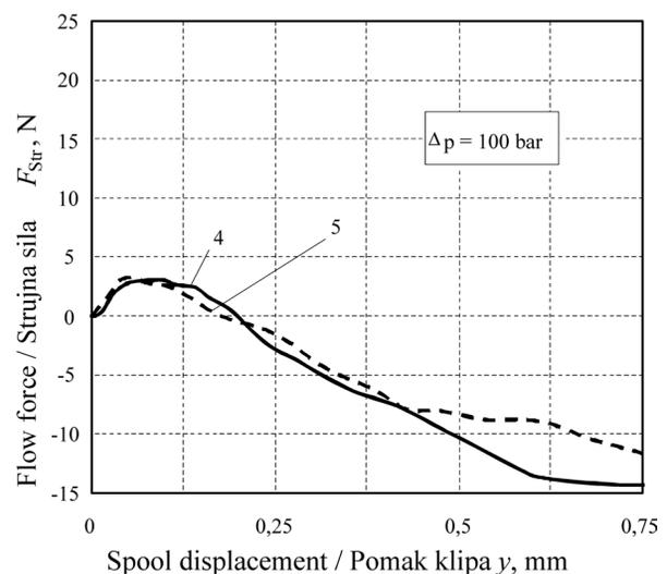
**Figure 14.** Flow-force measuring results, spool Nr. 4 and 5,  $\Delta p = 100$  bar, outlet edge (B- > T, A- > T)
