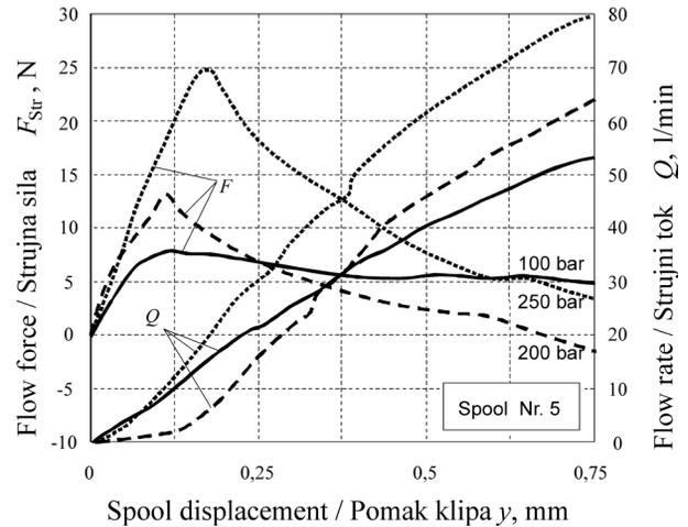
**Figure 13.** Flow-force measuring results, spool Nr. 5, the whole valve (P- > B- > A- > T)
