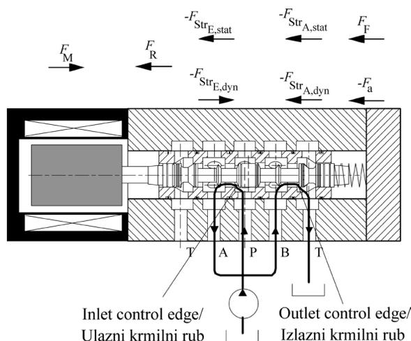
**Figure 1.** Forces acting on the valve spool (4-chamber structure)
