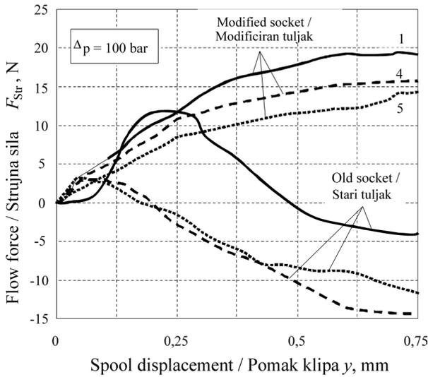
**Figure 15.** Flow-force measuring results, modified socket, valve piston Nr. 1, 4 and 5,  $\Delta p = 100$  bar, outlet edge (B- > T, A- > T)
