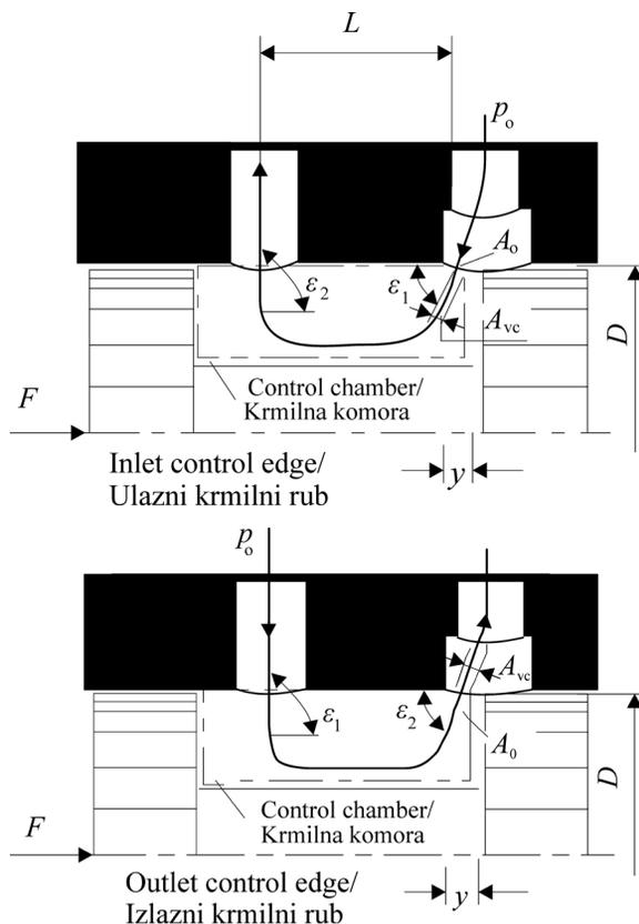
Figure 2. Flow forces acting on the valve spool
