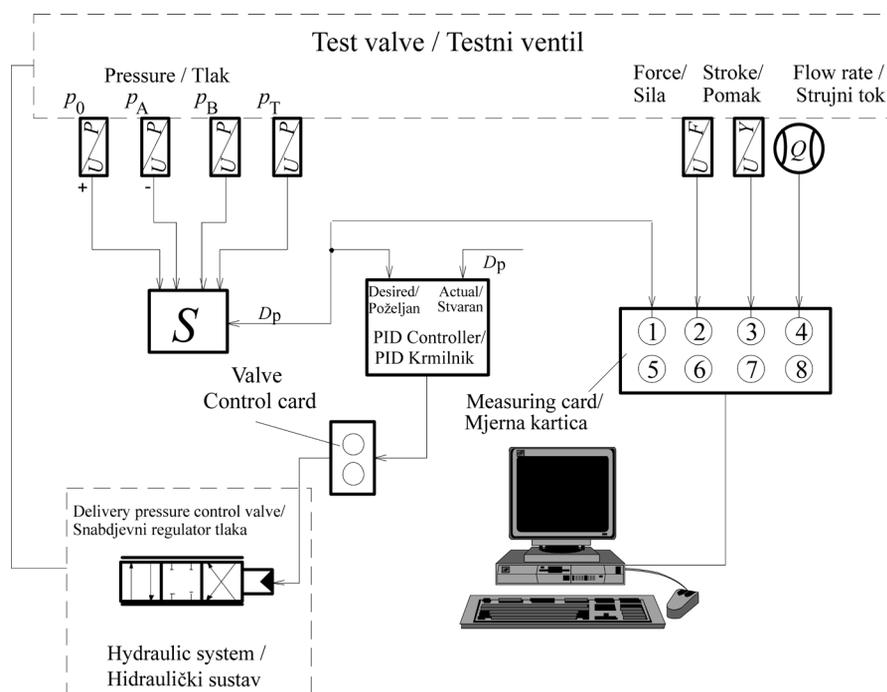
Figure 7. Test bench for measuring flow forces
