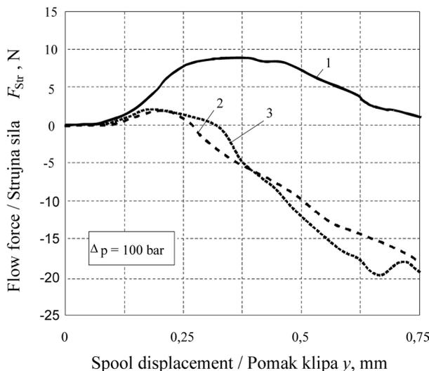
**Figure 10.** Flow-force measuring results, spool Nr. 1, 2 and 3,  $\Delta p = 100$  bar, inlet edge (P- > A, P- > B)
