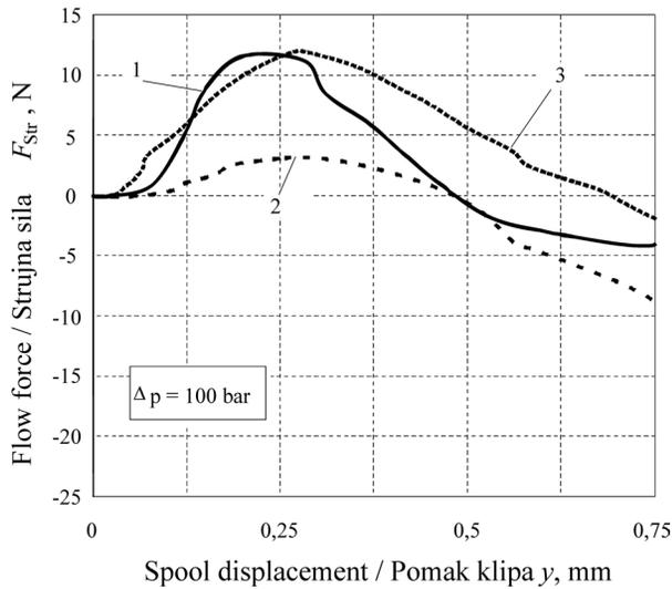
**Figure 11.** Flow-force measuring results, spool Nr. 1, 2 and 3,  $\Delta p = 100$  bar, outlet edge (A- > T, B- > T)
