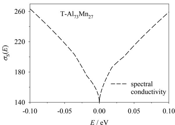
**Figure 4.** The spectral conductivity  $\sigma_s(E)$  for the T- $\text{Al}_{73}\text{Mn}_{27}$ . The singularity around the Fermi energy ( $E = 0$ ) is clearly pronounced. The sharpness of the pseudogap is directly related to the convex behavior of the electric conductivity,  $\sigma(T)$ , at low temperatures. The symmetric part clearly dominates the spectral function.
