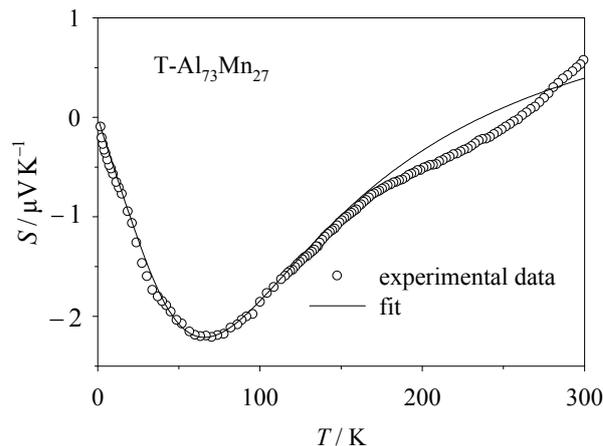
**Figure 2.** Thermoelectric power versus temperature for T-Al<sub>73</sub>Mn<sub>27</sub>. The experimental data are represented by circles. The full line is the result of the spectral conductivity modeling, as presented in the text.
