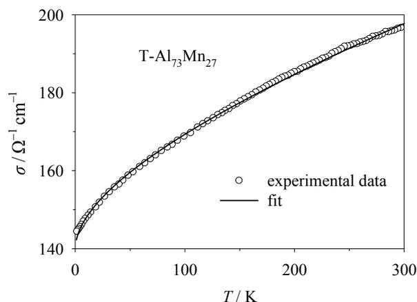
**Figure 1.** The electrical conductivity of T-Al<sub>73</sub>Mn<sub>27</sub> versus temperature. The circles represent the experimental data. The full line represents the fit discussed in the text.
