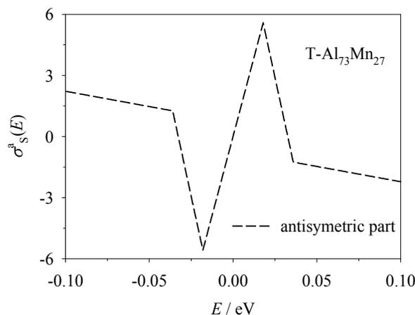
**Figure 3.** The antisymmetric part of spectral conductivity for the binary system T- $\text{Al}_{73}\text{Mn}_{27}$ . The advantage of this parameterization is direct interpretation of the model parameters as the widths of the characteristic windows in energy with characteristic values of  $\sigma_s^a(e)$  within these windows.
