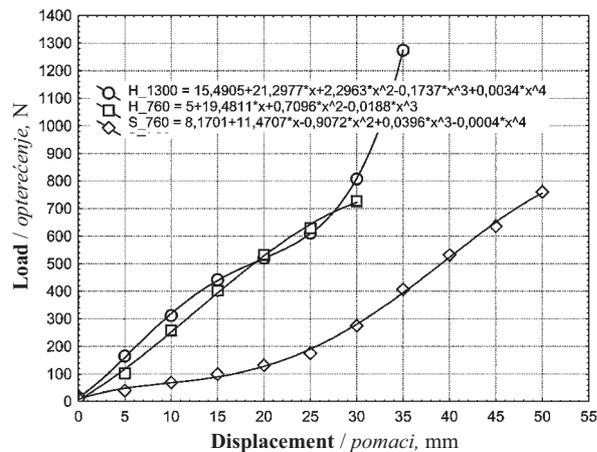
Figure 6 Seat cushion stiffness: H\_1300 – hard loading pad loading up to 1300 N, H\_760 – hard sensor, loading up to 760 N, S\_760 - soft loading pad loading up to 760 N
