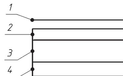
**Figure 1** Structure of the seat used in experiments: 1) upholstery fabric (1.5 mm thick), 2) cotton wool 120 g/m<sup>2</sup>, 3) T4060 polyurethane foam (40 mm thick), 4) particleboard (16 mm thick)
