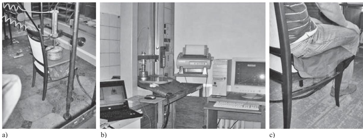
**Figure 3** Stands for seat cushion stiffness tests and contact pressures on their surface: a) a special testing machine developed for furniture certification, b) ZWICK 1445 testing machine, c) volunteer weighing 74 kg
