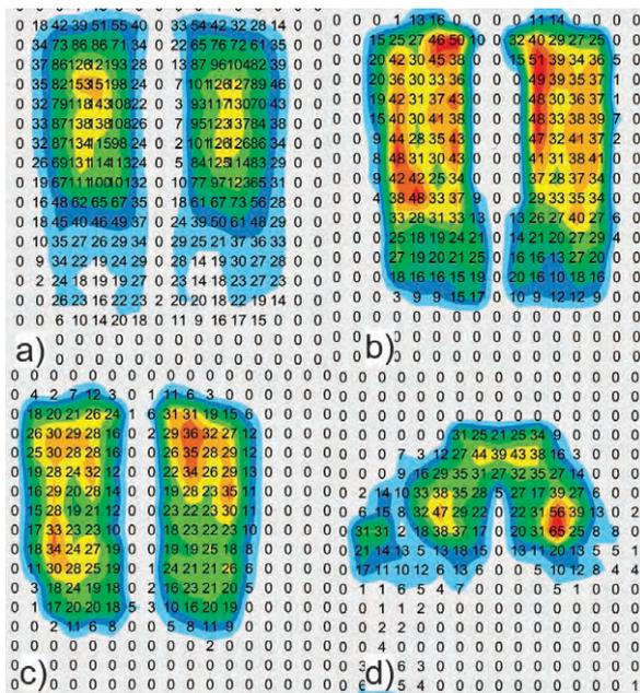
**Figure 7** Pressure distribution on the seat cushion surface in mmHg caused by: a) hard loading pad at the load of 1300 N, b) hard loading pad at the load of 760 N, c) soft loading pad at the load of 760 N, d) a volunteer of 74 kg weight
