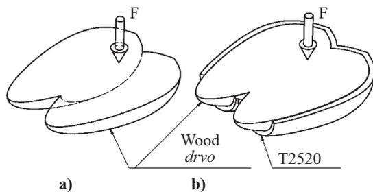
**Figure 2** Construction of the sensor used in investigations: a) hard, b) soft with 30 mm thick T4060 polyurethane foam
