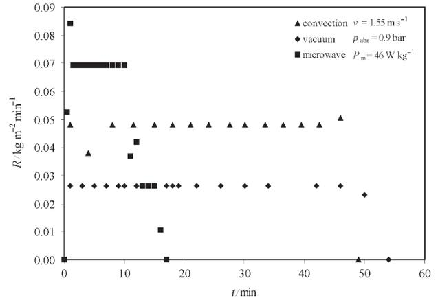
Fig. 8 – The effect of the heating mode on the drying kinetics ( $x = 1180\text{--}2360 \text{ }\mu\text{m}$ ,  $\vartheta = 60 \text{ }^\circ\text{C}$ )
