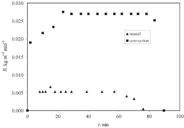
Fig. 7 – Drying rate curves for convective drying ( $v = 1.55 \text{ m s}^{-1}$ ,  $\vartheta = 40 \text{ }^\circ\text{C}$ ,  $x = 1180\text{--}2360 \text{ }\mu\text{m}$ ) (vertical and horizontal (tunnel) driers)
