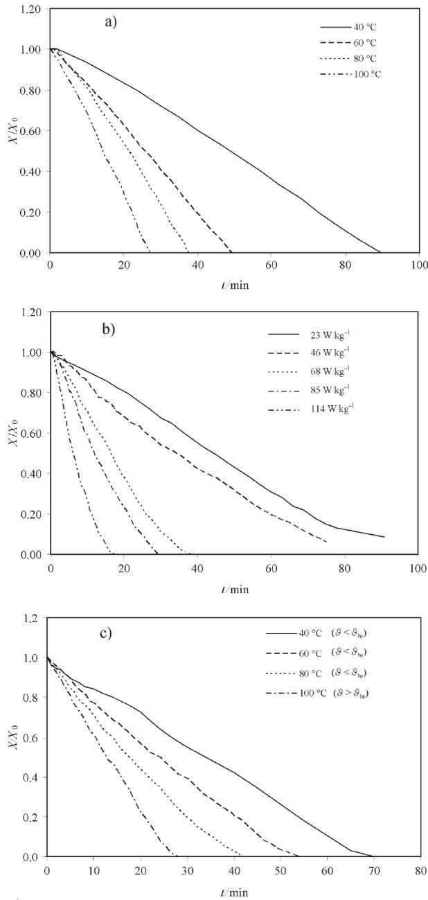
Fig. 3 – The influence of the heating intensity ( $x = 1180\text{--}2360 \mu\text{m}$ ) a) Convective drying ( $v = 1.55 \text{ m s}^{-1}$ ), b) Microwave drying, c) Vacuum drying ( $p_{\text{abs}} = 0.9 \text{ bar}$ )
