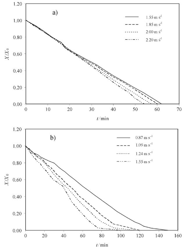
Fig. 4 – The influence of the hot air superficial velocity a) Convective drying ( $x = 600\text{--}850 \mu\text{m}$ ;  $\vartheta = 60 \text{ }^\circ\text{C}$ ), b) Tunnel drying ( $x = 1180\text{--}2360 \mu\text{m}$ ;  $\vartheta = 40 \text{ }^\circ\text{C}$ )
