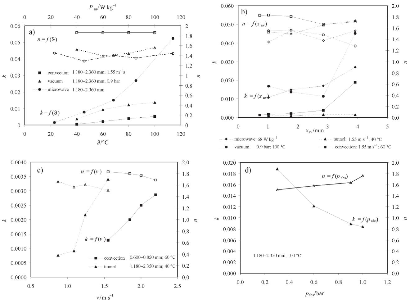
Fig. 10 – The influence of the operational conditions on the Page model parameters  $k$  and  $n$ : a) the influence of heating intensity, b) the influence of the particle size, c) the influence of the superficial air velocity, d) the influence of pressure
