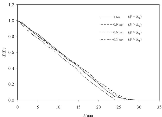
Fig. 5 – Vacuum drying: the influence of the pressure in the drying chamber ( $x = 1180\text{--}2360\ \mu\text{m}$ ;  $\vartheta = 100\ \text{°C}$ )
