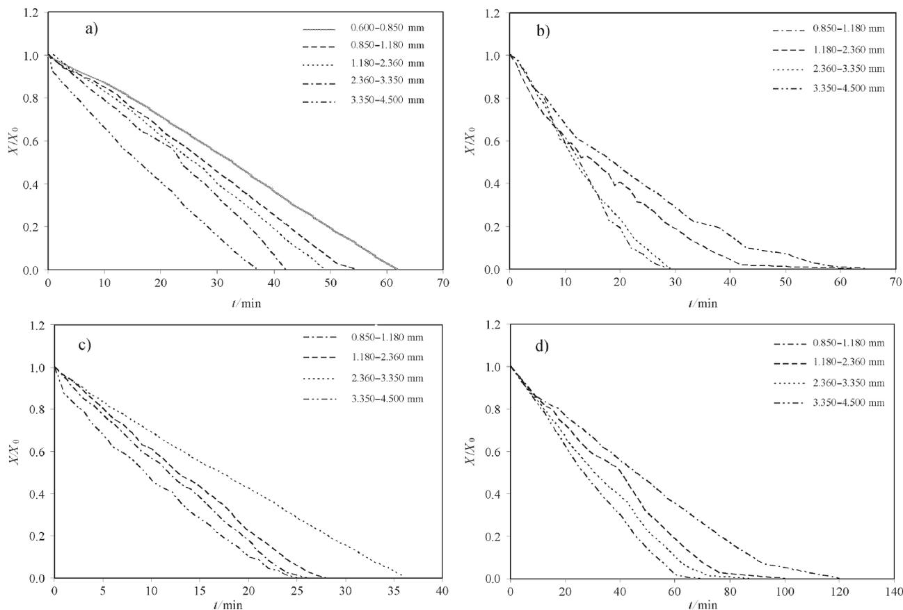
Fig. 6 – The influence of the particle size: a) Convective drying ( $v = 1.55\ \text{m s}^{-1}$ ;  $\vartheta = 60\ \text{°C}$ ), b) Microwave drying ( $P_m = 85\ \text{W kg}_{dm}^{-1}$ ), c) Vacuum drying ( $p_{abs} = 0.9\ \text{bar}$ ;  $\vartheta = 100\ \text{°C}$ ), d) Tunnel drying ( $v = 1.55\ \text{m s}^{-1}$ ;  $\vartheta = 40\ \text{°C}$ )
