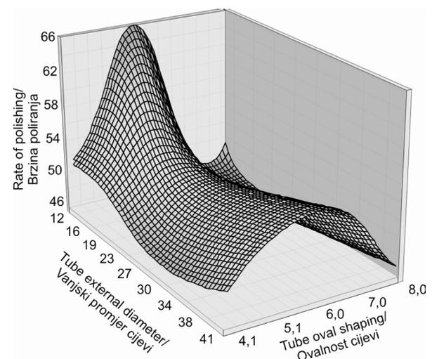
Figure 1. Functional dependence of the rate of polishing on outside diameter and oval shape of the tube
