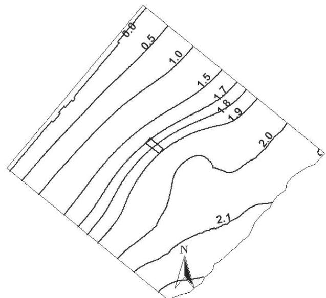
Figure 7A: Simulated groundwater levels in steady state conditions.
