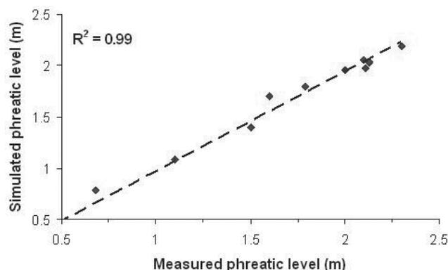
Figure 5: Comparison of measured and calculated groundwater levels.
