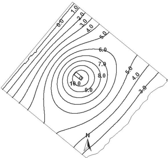
Figure 7C: simulated groundwater levels with infiltration after 365 days
