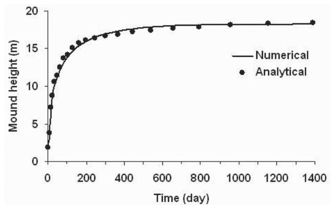
Figure 8: Comparison of numerical and analytical results.
