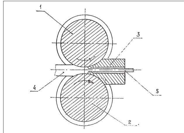
**Figure 7** Setup for continuous pressing by the Extrolling process [17,18]: 1-upper roll with groove; 2-bottom roll with groove; 3- matrix; 4- semifinished product; 5- finished product
