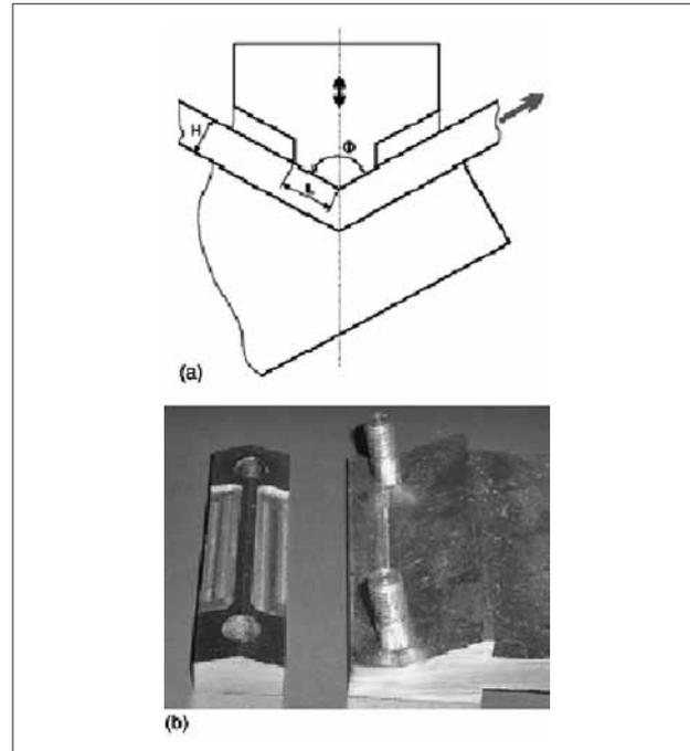
**Figure 11** Principal scheme of sheet processing by ECADS (a) and general view of the plunger and the base of the ECADS setup (b) [23]
