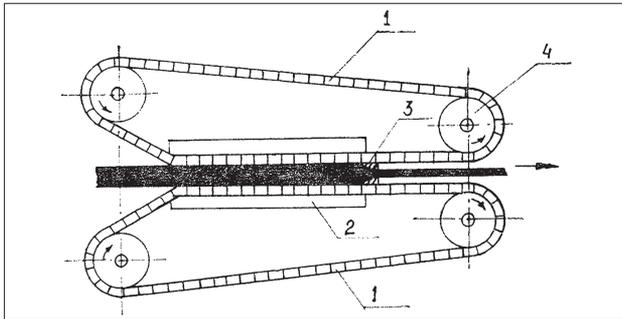
**Figure 5** Setup for continuous pressing by the Linex process [12-14]: 1-caterpillar chains; 2- guide member; 3- matrix; 4-cogwheels
