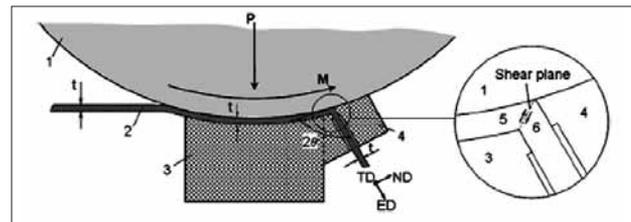
**Figure 4** Scheme of the CFAE setup [11]: 1-driving roll; 2- sheet workpiece; 3- workpiece support block; 4 - die assembly, where  $2\theta$  is the extrusion angle; 5- first extrusion channel; 6- second extrusion channel. (ED is the extrusion direction; ND is the normal to the sheet; TD is the transverse direction.)
