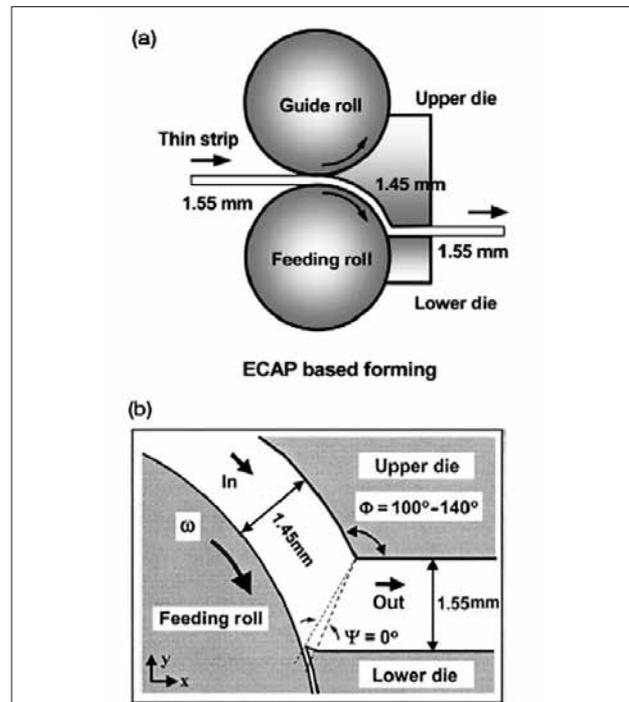
**Figure 8** (a) Schematic illustration of C2S2 continuous process based on ECAP for producing the metallic sheets. (b) A detailed die configuration of the forming zone in (a) [19]
