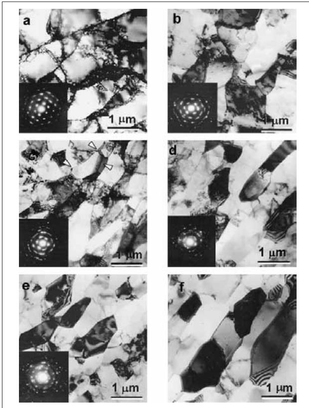
**Figure 9** TEM micrographs of Al alloy AA1050 after C2S2 at room temperature at an angle of  $120^\circ$  between the channels: (a)  $N=1$  ( $e=0,6$ ), (b)  $N=2$  ( $e=1,2$ ), (c)  $N=3$  ( $e=1,7$ ), (d)  $N=5$  ( $e=2,9$ ), (e)  $N=9$  ( $e=5,2$ ), and (f)  $N=50$  ( $e=29$ ) [19]
