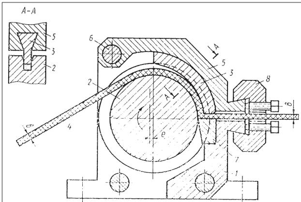
**Figure 2** Setup for continuous ECAP of long billets [8,9]: 1- case; 2- square pass drive roll; 3- ring sector insert; 4- semifinished product; 5- jaw; 6- axis of rotation; 7- stopper; 8- wedge clamp
