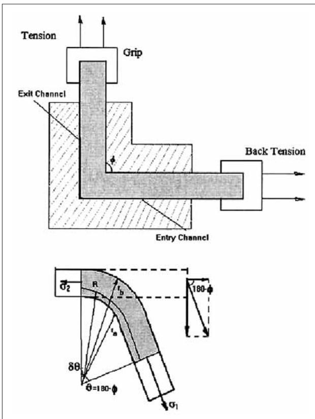
**Figure 10** Schematic illustration of drawing through the equal channel angular die [20-22]
