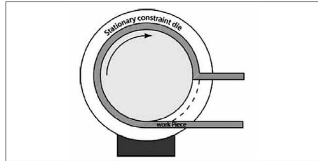
**Figure 3** Schematic illustration of the ECAP – Conform setup [10]
