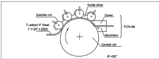
**Figure 6** Schematic illustration of the Conshearing process [15,16]
