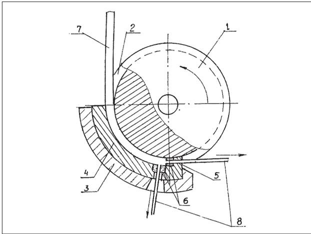
**Figure 1** Setup for continuous pressing by the Conform process [6,7]: 1-driving wheel; 2- ring groove; 3- shoe; 4- ring insert; 5- stopper; 6- matrix; 7- semifinished product; 8- finished product
