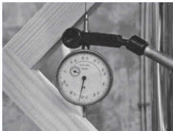
**Figure 7** Laboratory measurement of the joint edge point displacement
