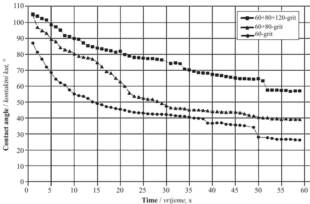
**Figure 4** Typical time-dependent contact angles of the MDF samples sanded with different sizes of sand paper grit
