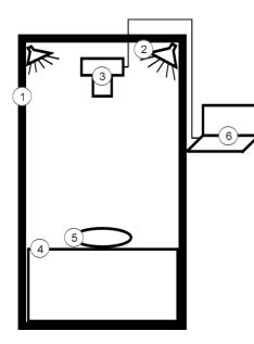
area of 760±5 Lux), digital camera (Panasonic Lumix DMC-FZ30) and software for image pre-processing and analysis (IrfanView, Adobe Photoshop, Global Lab Image/2). Apple discs for imaging were placed at 60 cm from camera.
