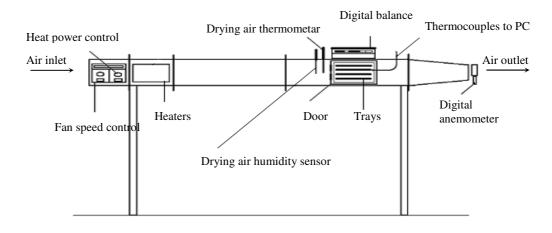
Fig. 1. Laboratory dryer used for convective drying
