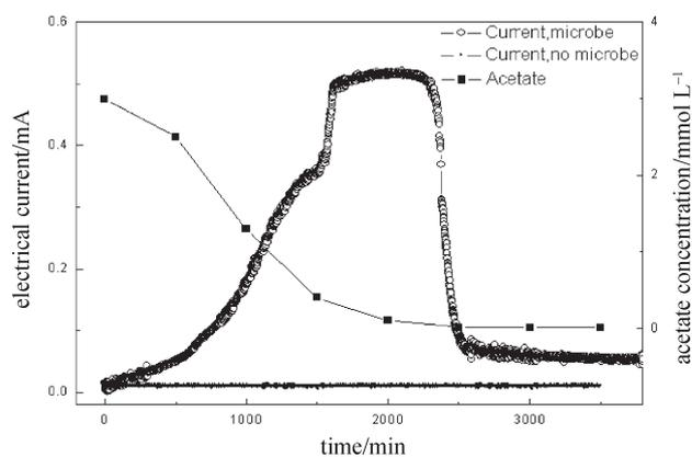
Fig. 3 – Current generation and acetate consumption during biofilm formation on the electrode
