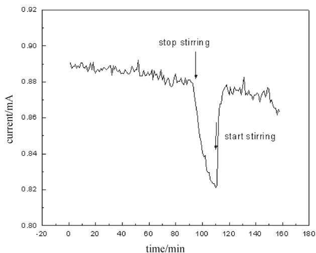
Fig. 7 – Effect of stirring on the current production of the MFC
