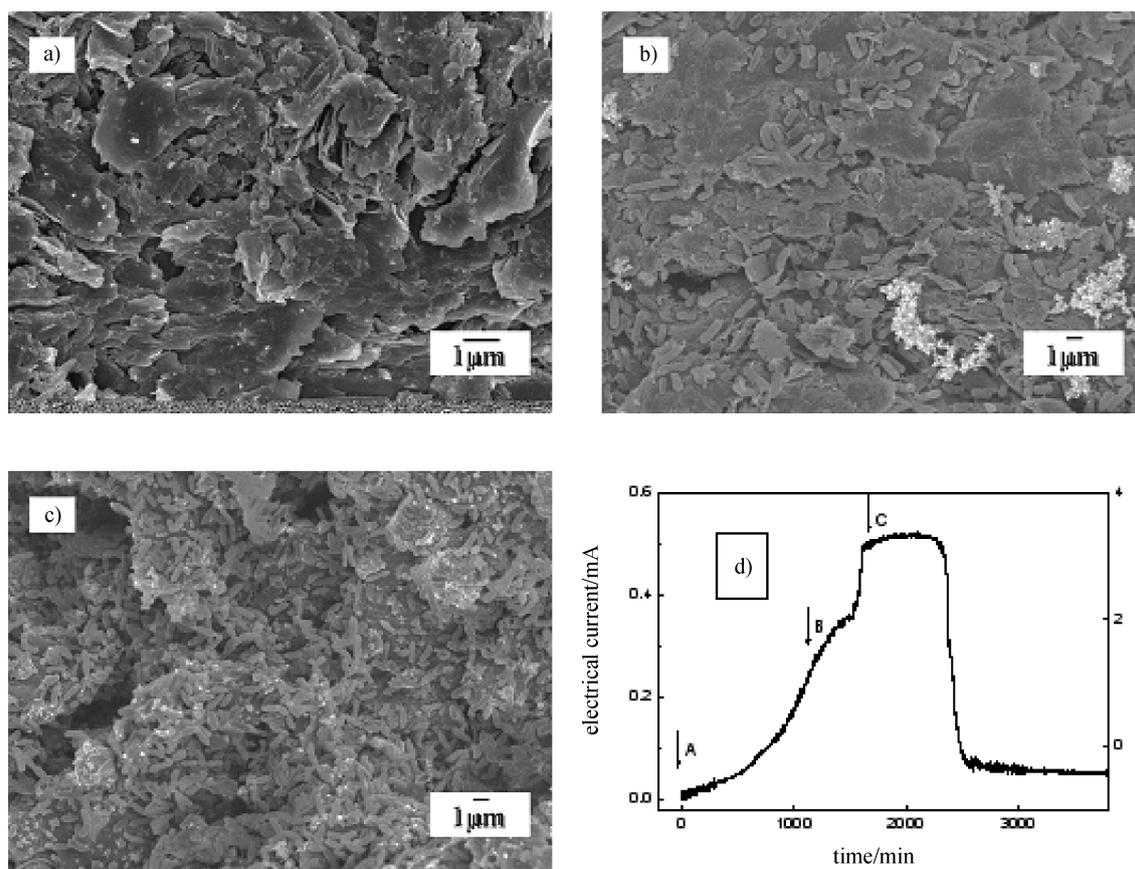
Fig. 1 – SEM images of an electrode surface at different times after inoculation into the anode: a) at the beginning of inoculation; b) 20 h after inoculation; c) the time when voltage became constant; d) current generation during biofilm formation
