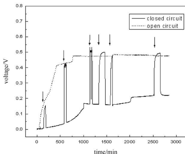
Fig. 6 – Time-voltage of the MFC with open and closed circuit (the closed circuit was disconnected as indicated by the arrows)
