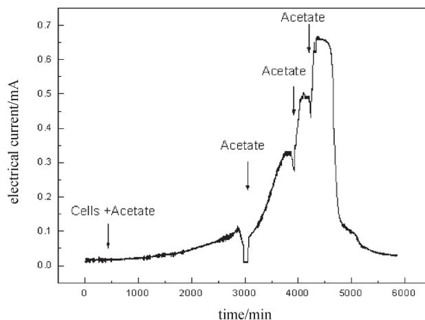
Fig. 5 – Current production by *G. metallireducens* when pulses of  $1 \text{ mmol L}^{-1}$  acetate were given at the indicated times
