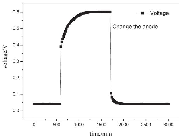
Fig. 4 – Voltage of MFC when the anode was changed
