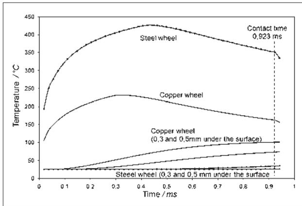
**Figure 4** Steel and copper wheel temperature profile under melt puddle as a function of contact time ( $u_w = 18,9\text{ m/s}$ , ribbon thickness  $66\mu\text{m}$ , contact time  $0,923\text{ msec}$ ,  $\alpha = 10^6\text{ W}/(\text{m}^2\cdot\text{K})$ )
