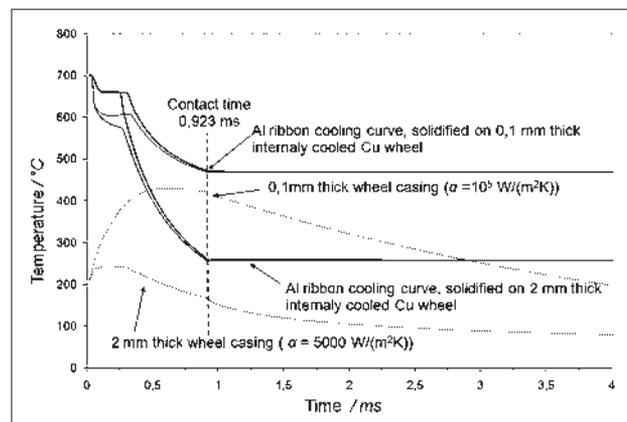
**Figure 6** Internally cooled copper wheel surface temperature increase as a function of contact time and thickness of wheel casing for aluminum casting ( $R_w = 0,2\text{ m}$ ,  $u_w = 18,9\text{ m/s}$ , ribbon thickness  $66\mu\text{m}$ , contact time  $0,923\text{ ms}$ )
