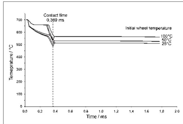
**Figure 5** Cooling curves for  $66\mu\text{m}$  thick Al ribbon as a function of initial wheel temperature and contact time ( $u_w = 18,9\text{ m/s}$ ,  $\alpha = f(x)$ )
