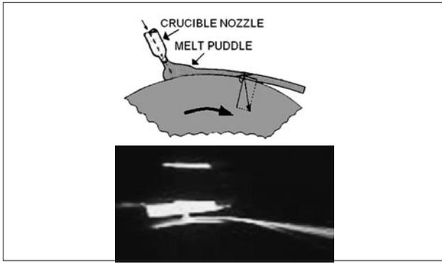
**Figure 1** Melt puddle formation on the surface of the chill wheel at free jet melt-spinning process [2]
