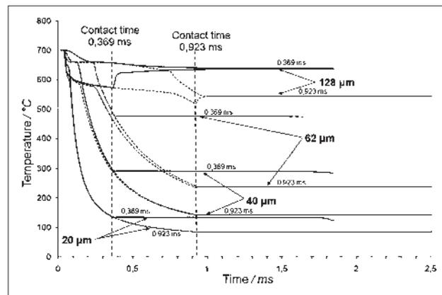
**Figure 3** Cooling curves of contact and free surface of aluminium ribbon as a function of its thickness and contact time ( $u_w = 18,9 \text{ m/s}$ ,  $\alpha = f(x)$ )
