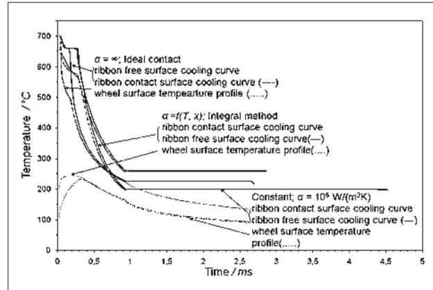
**Figure 2** Cooling curves of free and contact surface of Al ribbon and contact surface temperature profile of copper wheel as a function of different contact resistance assumption ( $u_w = 18,9 \text{ m/s}$ , ribbon thickness  $66 \mu\text{m}$ , contact time  $0,923 \text{ ms}$ )
