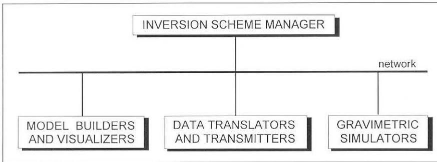
Fig. 3 Software architecture.
