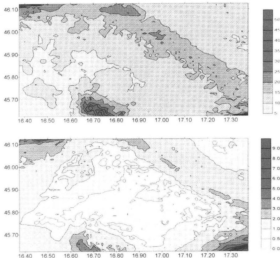
Fig. 5 a) Topographic correction from 3D density model (in  $10^{-5} \text{ ms}^{-2}$ ); b) deflections of vertical from 3D density model (in arcsec).
