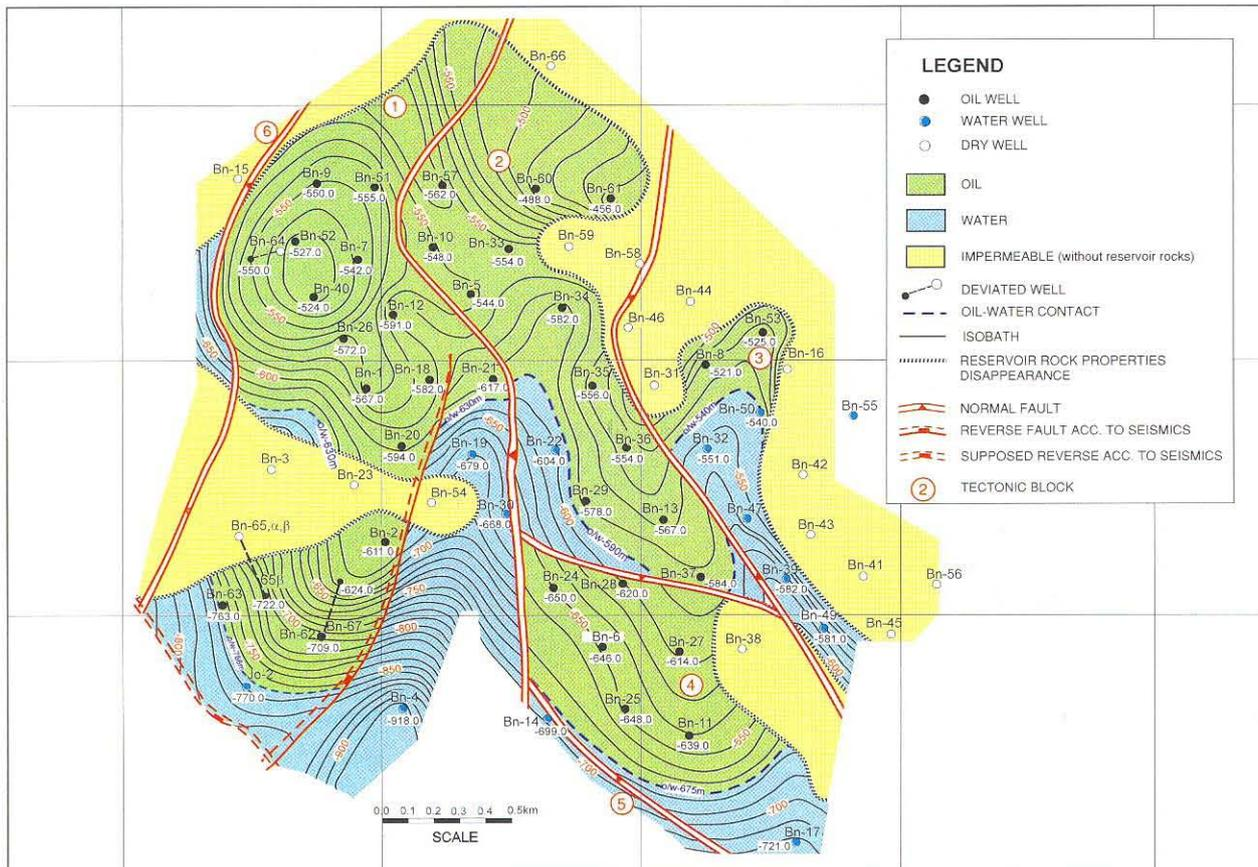
Fig. 4. Contour map of the top of the "V" reservoir.
