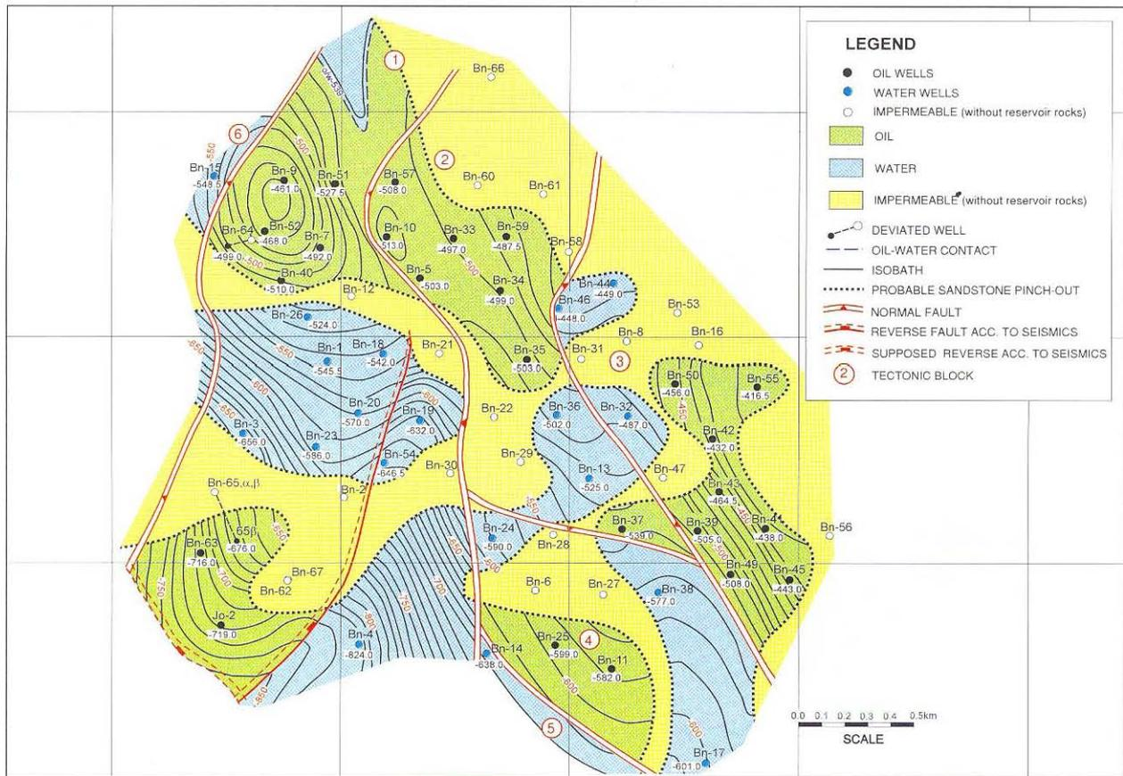
Fig. 3 Contour map of the top of the "III" reservoir.
