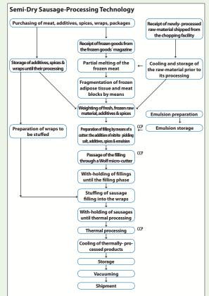
**Figure 1** The scheme outlines the technological production process, and points out the critical control points (CCPs)
