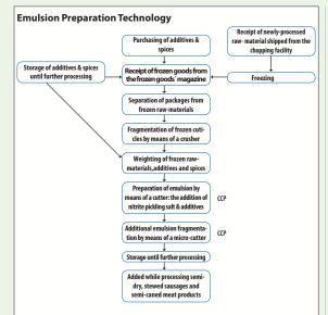
**Figure 2** The scheme outlines the technological production process, and points out the critical control points (CCPs)
