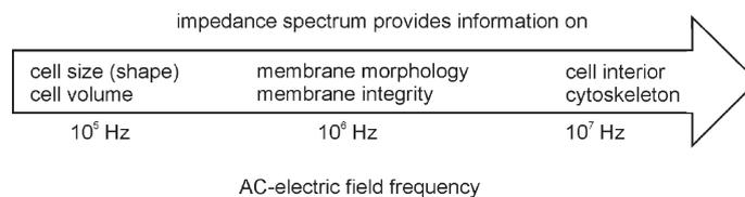
Fig. 7 – Impedance measurement for cell characterization: AC electric field frequencies and the detection of cell properties
