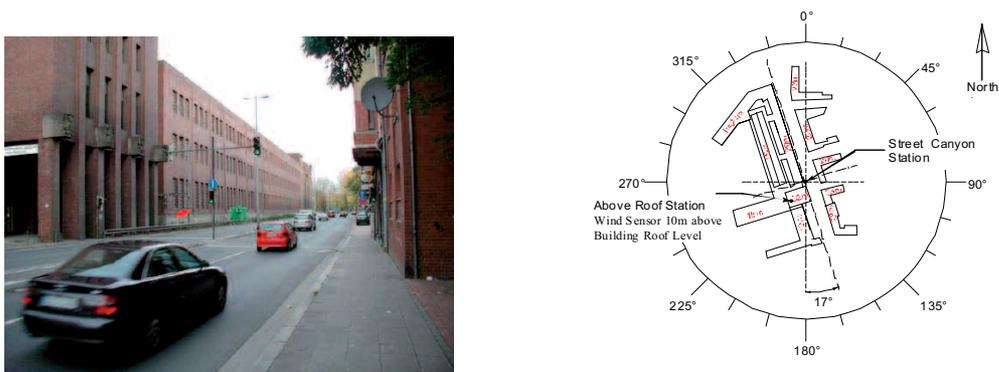
Figure 1. Experimental site and orientation of the street canyon towards the wind.
