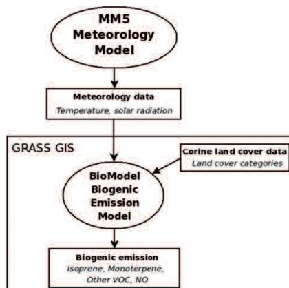
Figure 1. Diagram of biogenic emission modelling system.
