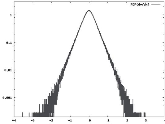
Figure 4. The PDF of the velocity gradient  $dv/dx$  for the ext. limiter in  $t = 40$ .
