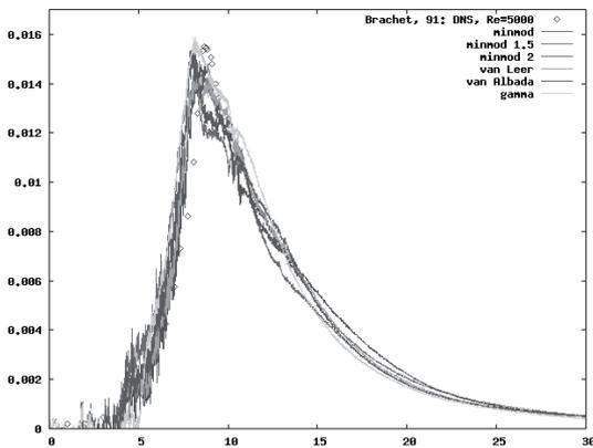
Figure 1. The kinetic energy dissipation for various limiters.
