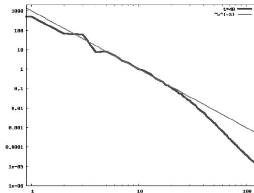
Figure 3. The kinetic energy spectrum in  $t = 40$  for ext. minmod limiter.
