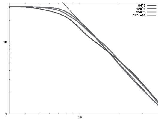
Figure 2. The time history of the kinetic energy for three resolutions for ext. minmod limiter.
