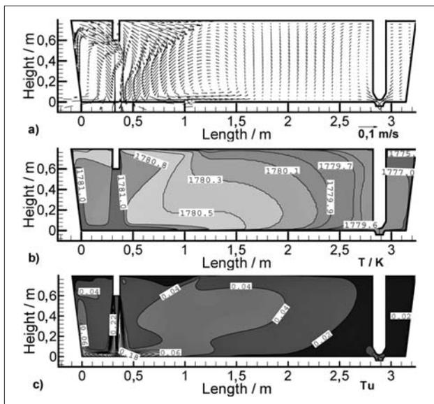
**Figure 5** Non-isothermal CFD predictions of the velocity, temperature and turbulence intensity distribution in an original tundish
