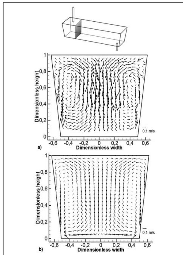
Figure 3 Velocity distribution at the plane  $x/L=0,2$ : a) measured with LDA, b) mathematically predicted
