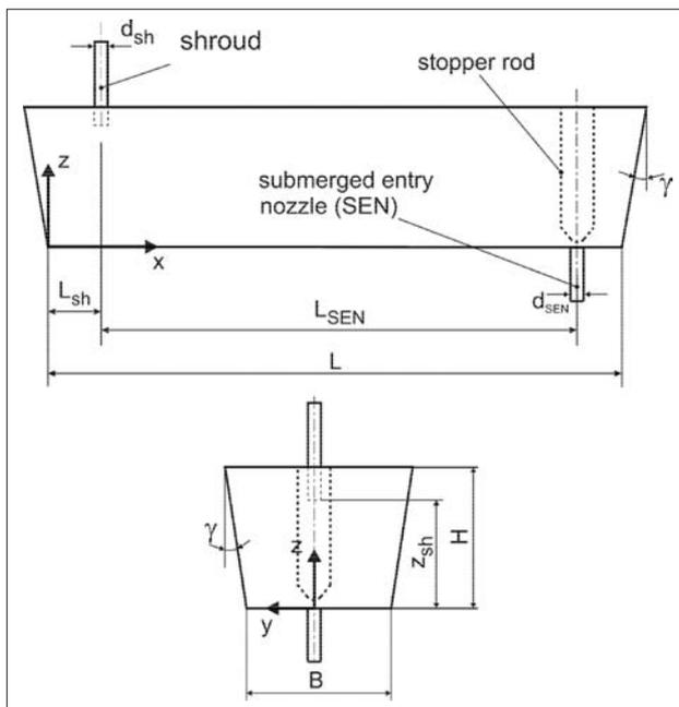
**Figure 1** Illustration of the shape and dimensions of the tundish
