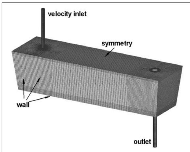
Figure 2 Structured mesh with boundary conditions used for the simulations
