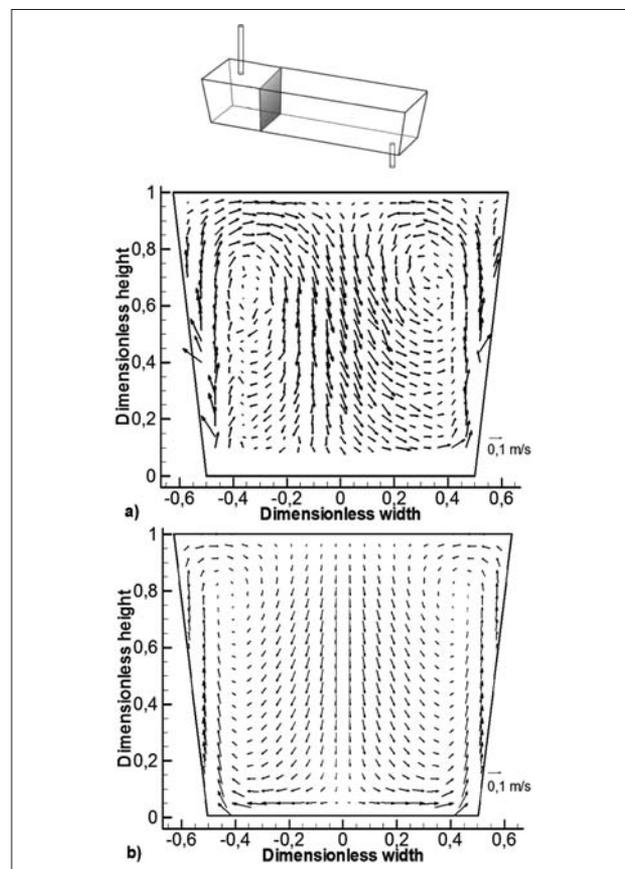
Figure 4 Velocity distribution at the plane  $x/L=0,3$ : a) measured with LDA, b) mathematically predicted
