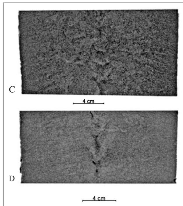
**Figure 5** Macrostructure image on longitudinal section of an ingot cast of high-carbon steel (samples C3 and D3); ingot C – with acoustic treatment; ingot D – without acoustic treatment.
