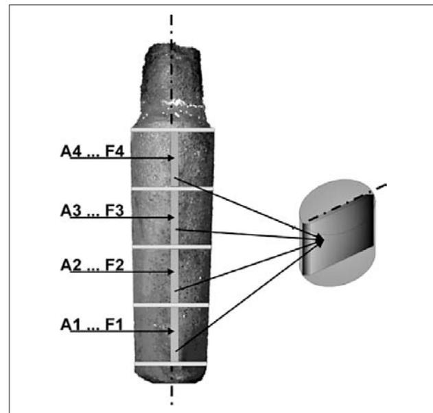
Figure 2 Diagram of longitudinal disk sampling from cast ingots.
