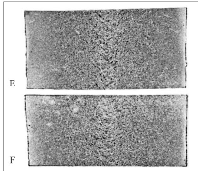
**Figure 4** Distribution of sulphur on the longitudinal section of high-carbon steel ingots (samples E3 and F3); ingot E – time of acoustic treatment 90 seconds; ingot F – time of acoustic treatment 300 seconds.
