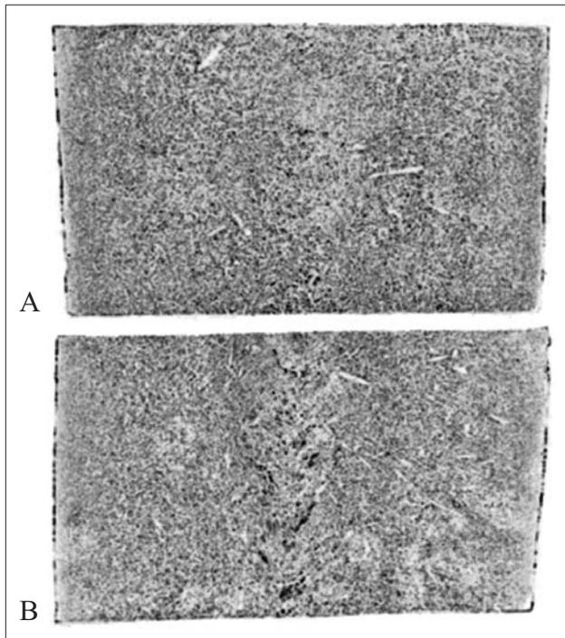
**Figure 3** Distribution of sulphur on longitudinal section of high-carbon steel ingots (samples A3 and B3); ingot A – with acoustic treatment; ingot B – without acoustic treatment.
