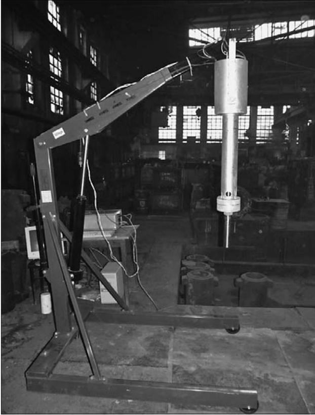
Figure 1 Experimental apparatus for acoustic treatment of ingots.
