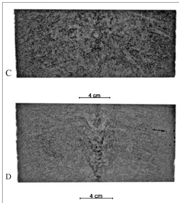
**Figure 6** Macrostructure image on longitudinal section of an ingot cast of high-carbon steel (samples C4 and D4); ingot C – with acoustic treatment; ingot D – without acoustic treatment.
