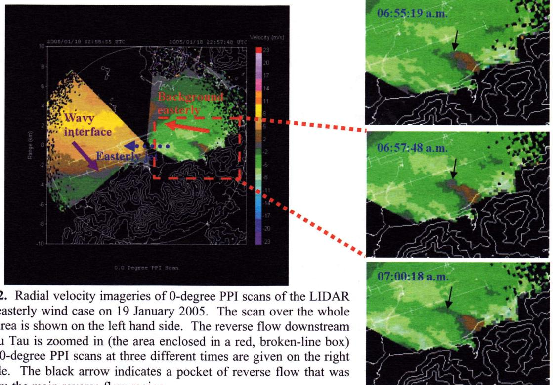
**Figure 2.** Radial velocity imageries of 0-degree PPI scans of the LIDAR for the easterly wind case on 19 January 2005. The scan over the whole airport area is shown on the left hand side. The reverse flow downstream of Lo Fu Tau is zoomed in (the area enclosed in a red, broken-line box) and the 0-degree PPI scans at three different times are given on the right hand side. The black arrow indicates a pocket of reverse flow that was shed from the main reverse flow region.
