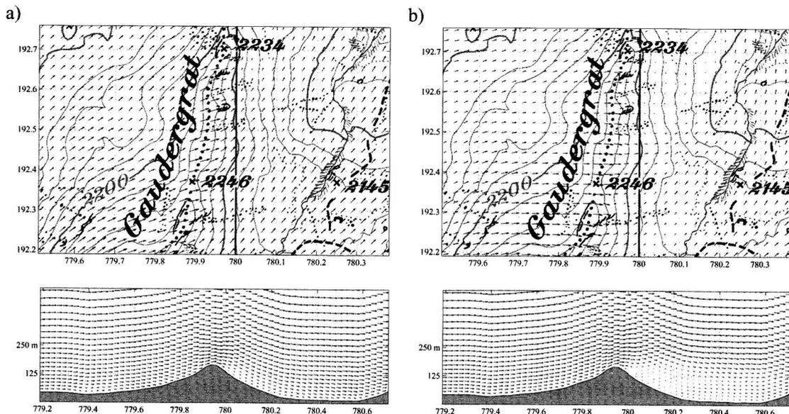
Figure 1. CFX-4; Top view and vertical cross section of the wind field over the Gaudergrat Ridge after 480 s simulation time. (Horizontal units are in the Swiss Official Coordinate System [km])
