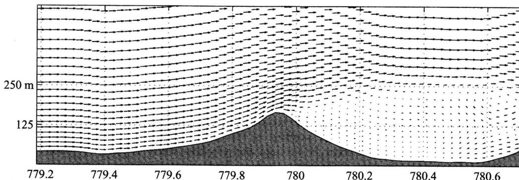
Figure 3. CFX-4; Separation eddy behind the ridge using inappropriate boundary conditions. The eddy becomes too large and extends to the entire valley located on the lee-side.
