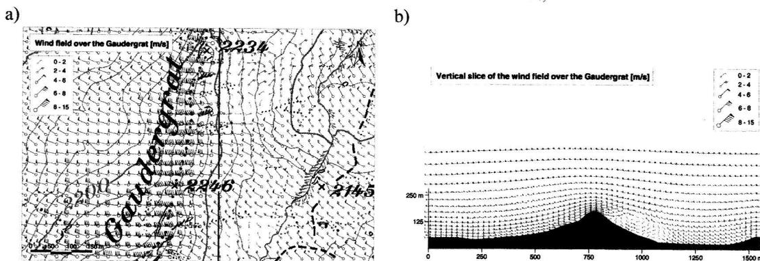
Figure 2. ARPS; a) Top view and b) vertical cross section of the wind field over the Gaudergrat Ridge after 480 s simulation time for West wind (270°). Situation similar to Figure 1 b).
