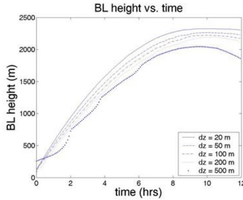
**Figure 1.** BL height evolution as estimated by the TM model, at different vertical resolutions ( $dz$ ); the surface heat flux  $H_0$  varies according to  $H_0 = H_{max} \sin \omega t$  (here  $2\pi\omega^{-1} = 24$  h,  $H_{max} = 0.2$  K m s<sup>-1</sup>).
