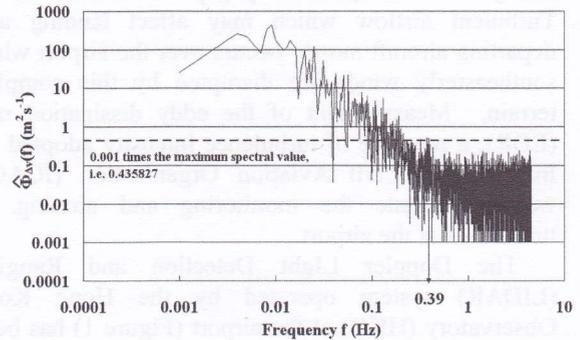
**Figure 2.** The spectrum  $\hat{\Phi}_{\Delta v}(f)$  between the range gates 3 km and 3.3 km from the LIDAR for a 12-minute period starting at 9:57 a.m., 28 August 2004. The frequency indicated by an arrow (0.39 Hz) corresponds to the point where 0.001 times of the maximum spectral value is first exceeded.
