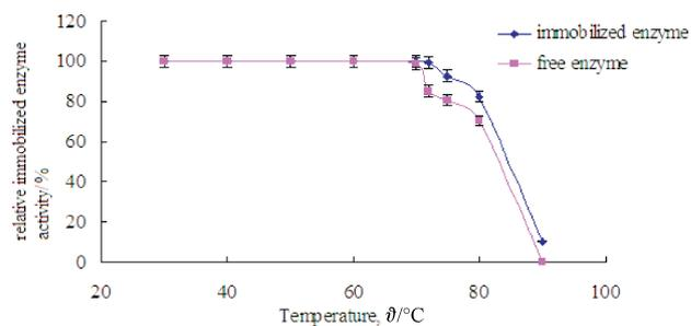
Fig. 10 – Temperature stability of free and immobilized enzyme
