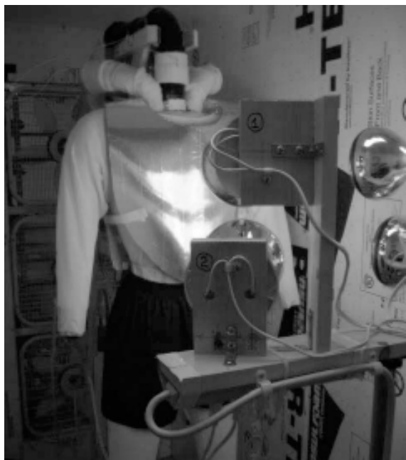
Figure 3. Illustration of the inflatable thermal manikin exposed to infrared heat radiation while wearing the prototype vest
