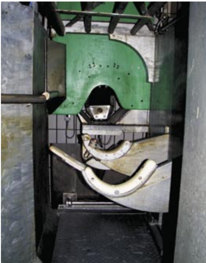
Fig. 3. Internal view of the stunning box (in animal direction): Breast and abdomen support bars (with cardio-electrode) and head fixing slide (green) in stunning position; muzzle electrode (centre back) (With the permission of BANSS, Biedenkopf, Germany)
