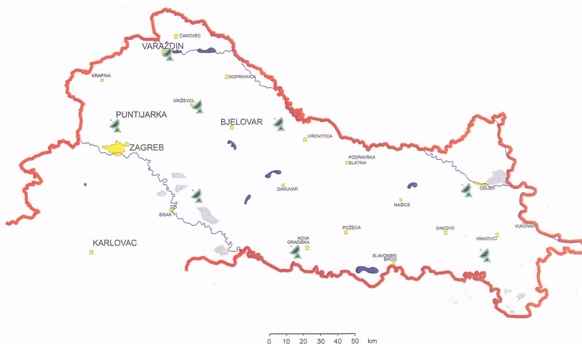
Figure 1. The region of the operational hail suppression project in Croatia and the meteorological stations. The points are the launching stations and the radar symbols are the radar stations.
