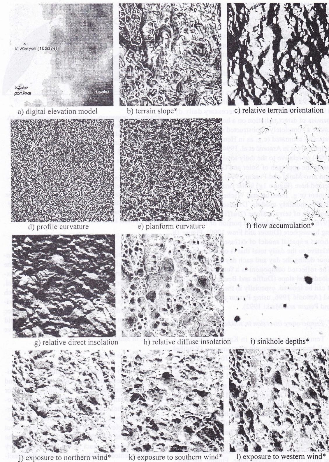
Figure 1. Examples of topoclimatic models for the central part of NP Risnjak (Croatia). Model values in the gray scale: black = minimum, white = maximum (\* reversely).
