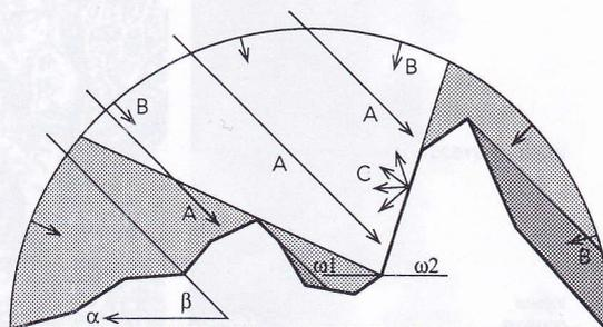
Figure 2. Components of incoming solar irradiance (A - direct irradiance, B - diffuse sky irradiance, C - irradiance reflected by nearby terrain) and some independent variables in the solar irradiance modelling ( $\alpha$  - Sun azimuth,  $\beta$  - Sun elevation,  $\omega$  - horizon elevation, elevation of the unobstructed part of the sky).
