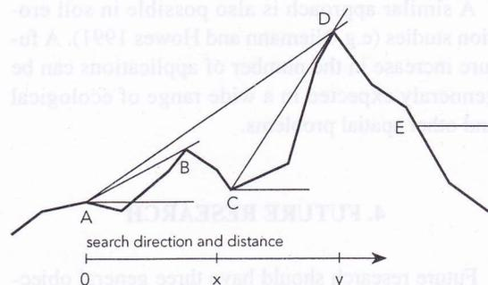
Figure 4. Some possible relations between search distance and horizon elevation: for point A - under distance 'x', the critical point is B, under distance 'y', the critical point is D; for point C - the critical point is D under both distances; for point E - the horizon elevation is set to zero.
