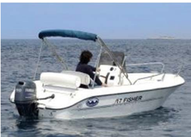
Slika 7. Brza brodice „Fisher“ s izvanbrodskim motorom pričvršćenim na krmenom zrcalu Figure 7. Skimming boat "Fisher" with outboard engine attached to the transom?
