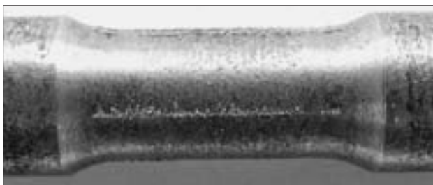
Figure 1 Fatigue test sample with longitudinal surface crack covered by titanium powder
